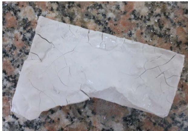
**Figure 10** Improper surface cracks
