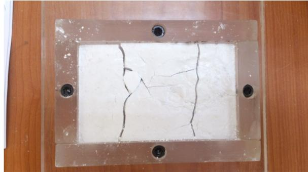
**Figure 8** Crack appearances in gelled ceramics
