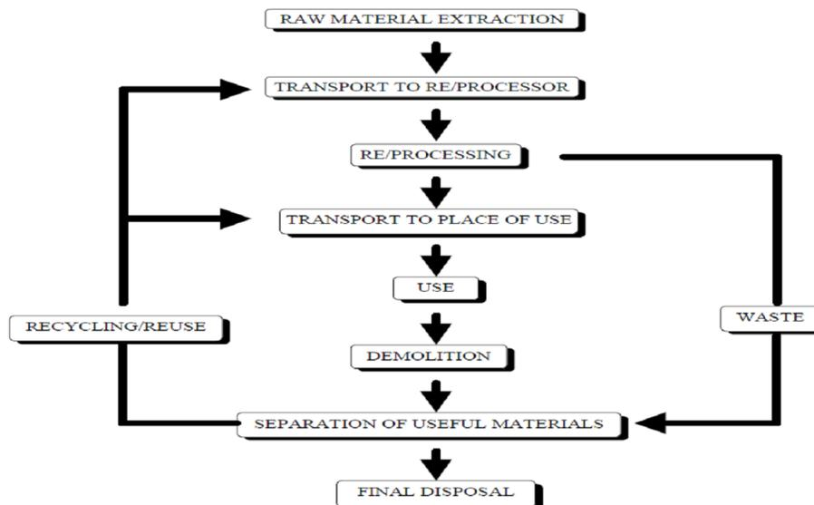
Fig. 3: Construction Materials Life-Cycle, Source: [24]
