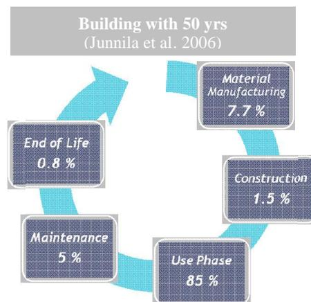
**Fig. 1: Environmental Impacts along Building Life -Cycle, Source: [20]**
