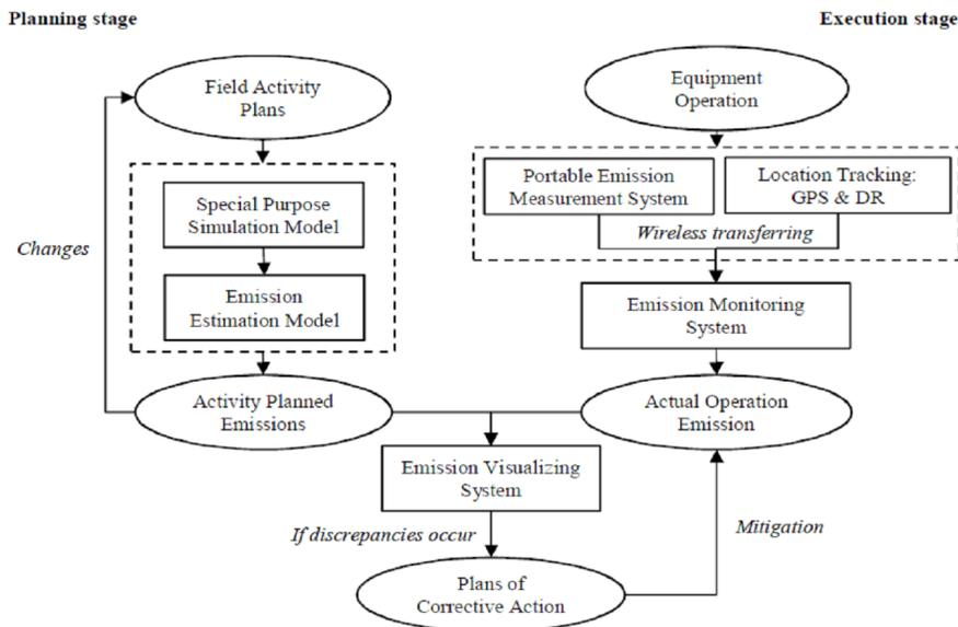
Fig. 5: Emission Management Framework for Construction Processes, Source: [20]
