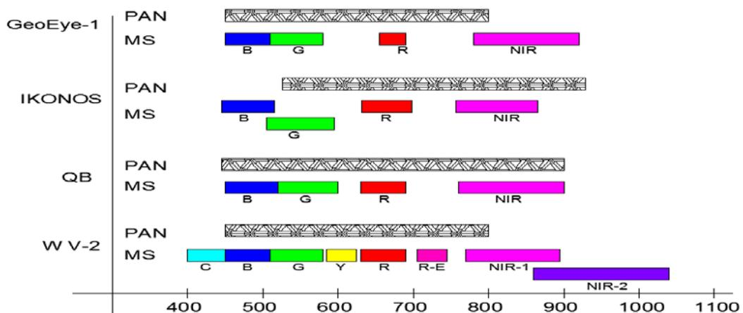
Figure 1 comparison between spectral band coverage of WV-2, QB, IKONOS and GeoEye-1
