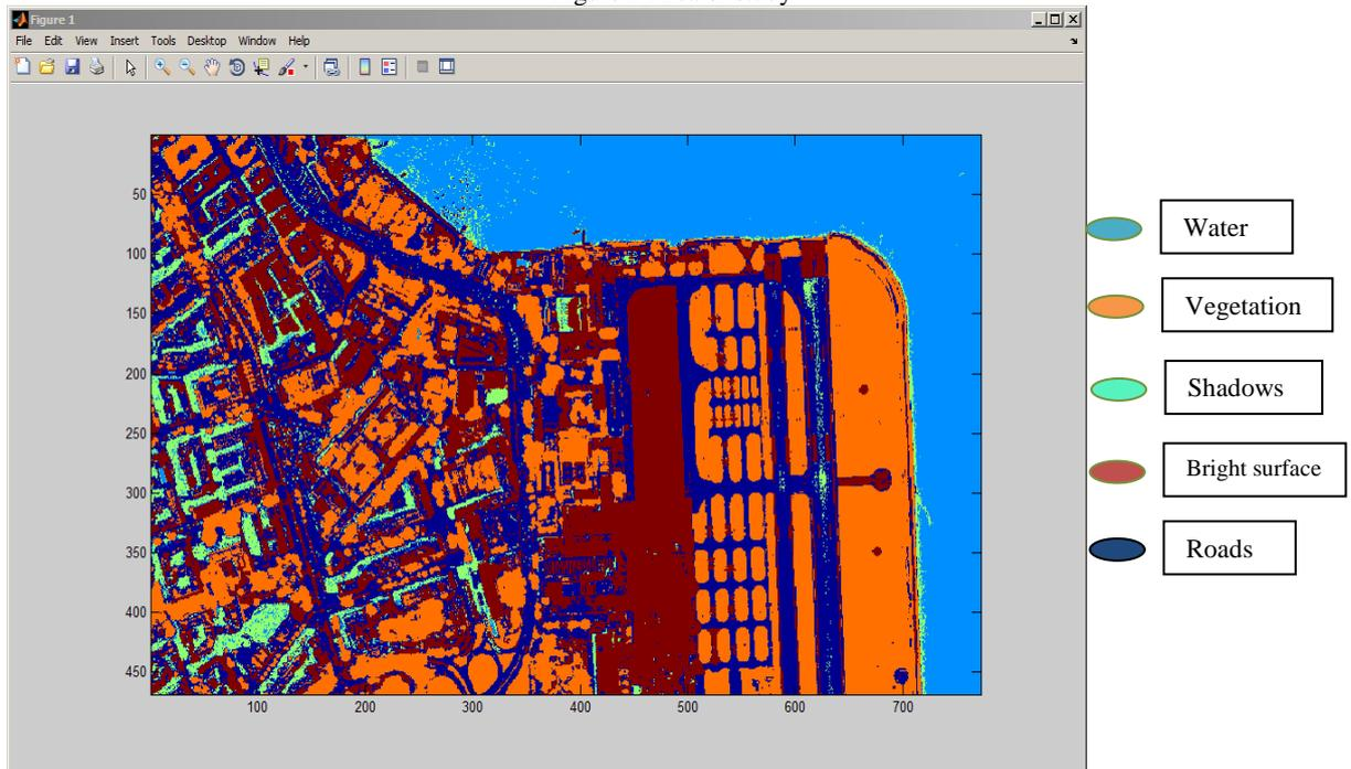
Figure 3 Classification results of the proposed modified parallelepiped method
