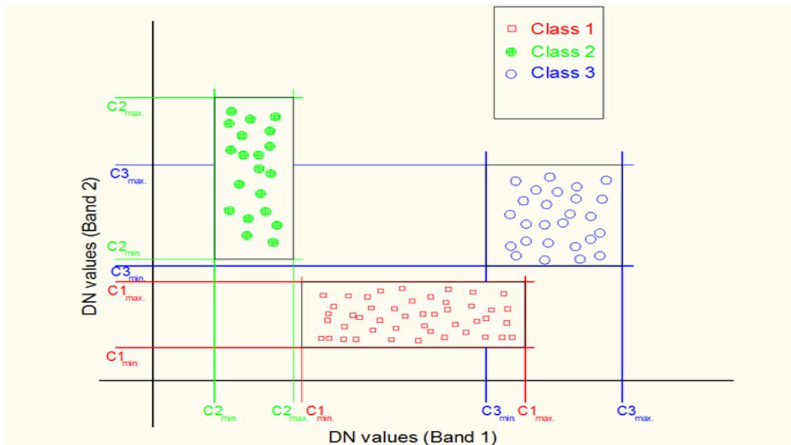
Figure 2 Implementation of the parallelepiped classification method for three classes using two spectral bands, after (Tso and Mather 2009)
