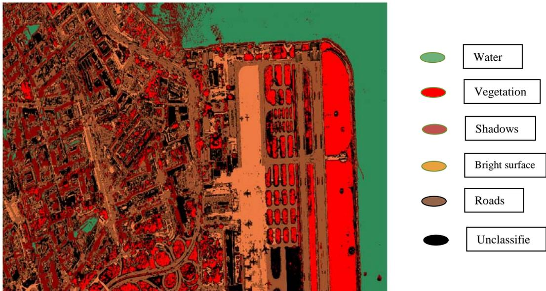
Figure 4 Classification results of the traditional parallelepiped method.
