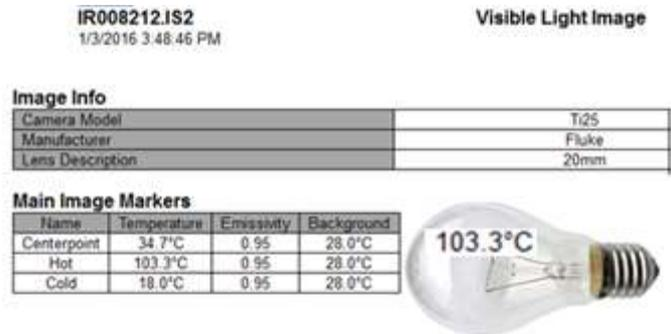
Fig.3. Measured temperature for 40w incandescent lamp
