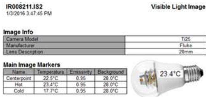
Fig.5. Measured temperature for 10w LED lamp
