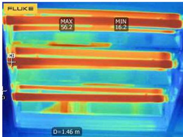
Fig.6. Measured temperature for fixture (3 x 60cm) fluorescent lamps
