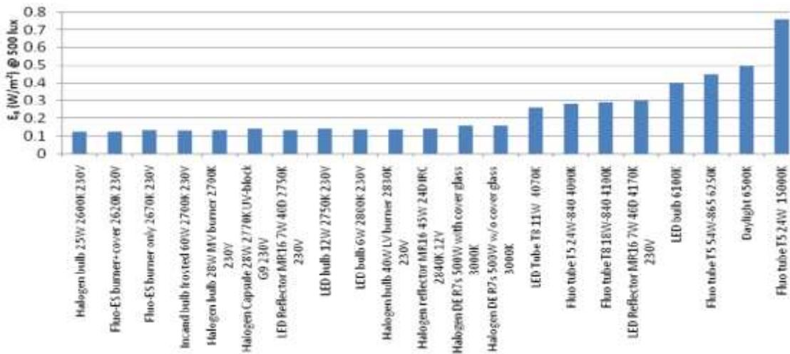
Fig(1) Comparison of various light sources on blue light hazard irradiance at 500 lux
