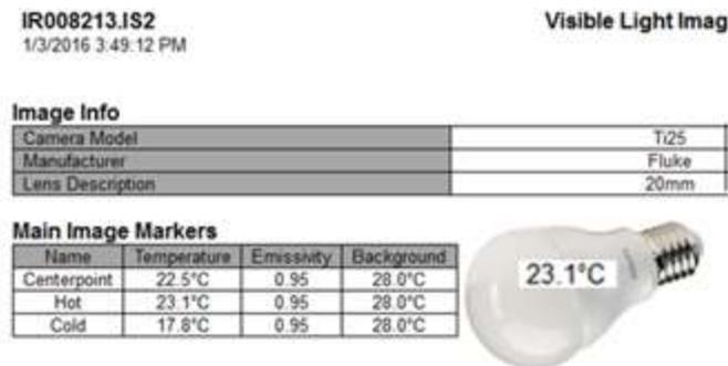
Fig.4. Measured temperature for 5.5w LED lamp
