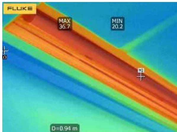
Fig.7. Measured temperature for LED fixture (2x 120cm)
