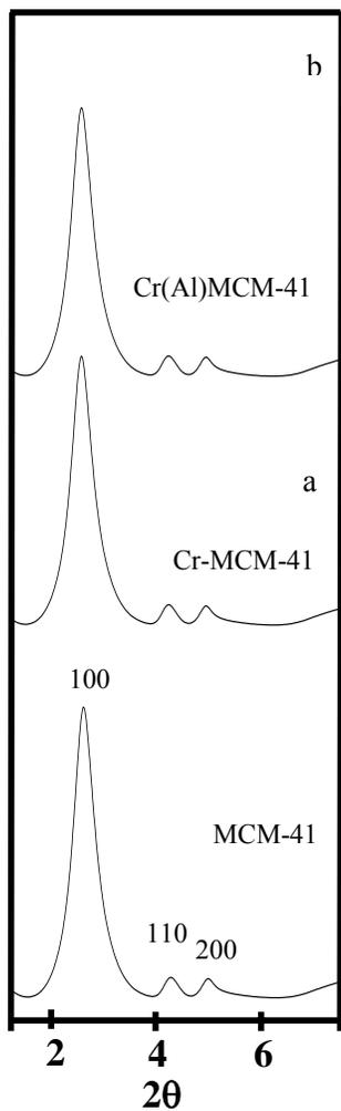
Fig. 1: XRD of MCM-41 in comparison with Cr-MCM-41 prepared by two different methods
