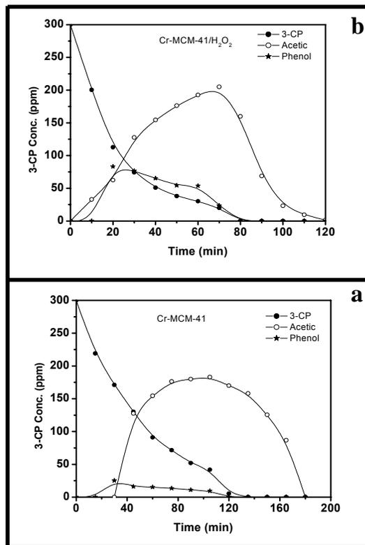
Fig. 8: Photodegradation of 3-CP and concomitant appearance of intermediate products formed during irradiation.
