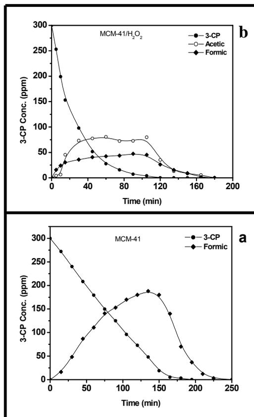
Fig. 6: Photodegradation of 3-CP and concomitant appearance of intermediate products formed during irradiation.
