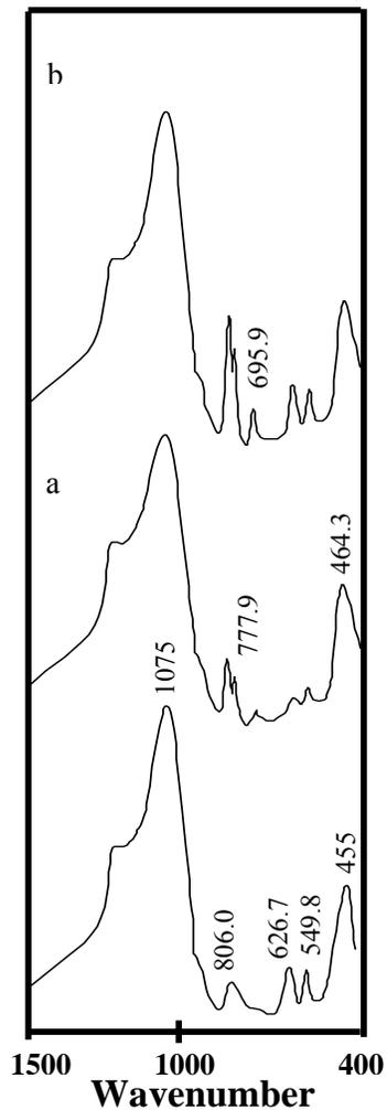
Fig. 2: FTIR spectra of MCM-41 in comparison with Cr-MCM-41 prepared by two different methods
