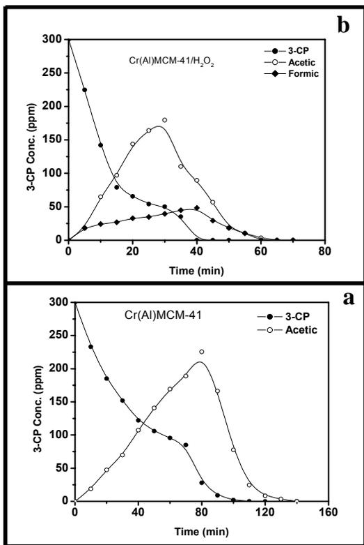
Fig. 7: Photodegradation of 3-CP and concomitant appearance of intermediate products formed during irradiation.
