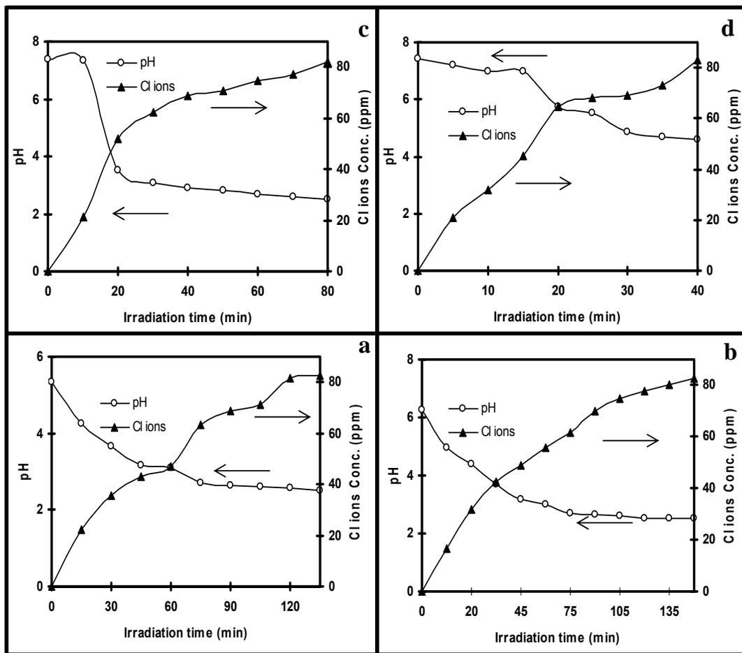
Fig. 10: Variation of chloride ions and pH during the photo-degradation process as a function of irradiation time.
