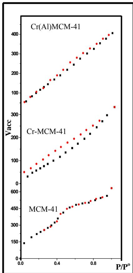
Fig. 3: Nitrogen adsorption-desorption isotherm of MCM-41 in comparison with that of Cr-MCM-41 prepared with two different methods.
