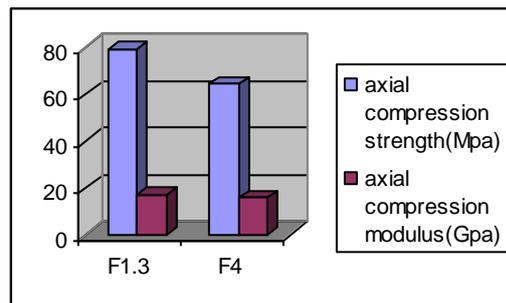
Figure 4: Comparison between mechanical properties of composite material based on CF/epoxy resin and composite material based on CF/phenolformaldehyde resin.
