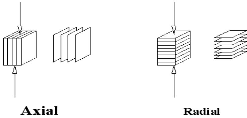
Figure 3: Axial and radial compression specimens for composite material
