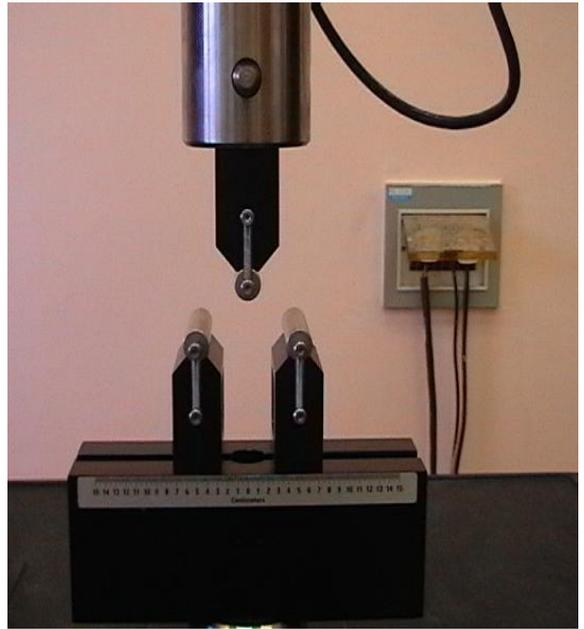
Figure 1: RT30 Material Testing System used for compression and flexural tests
