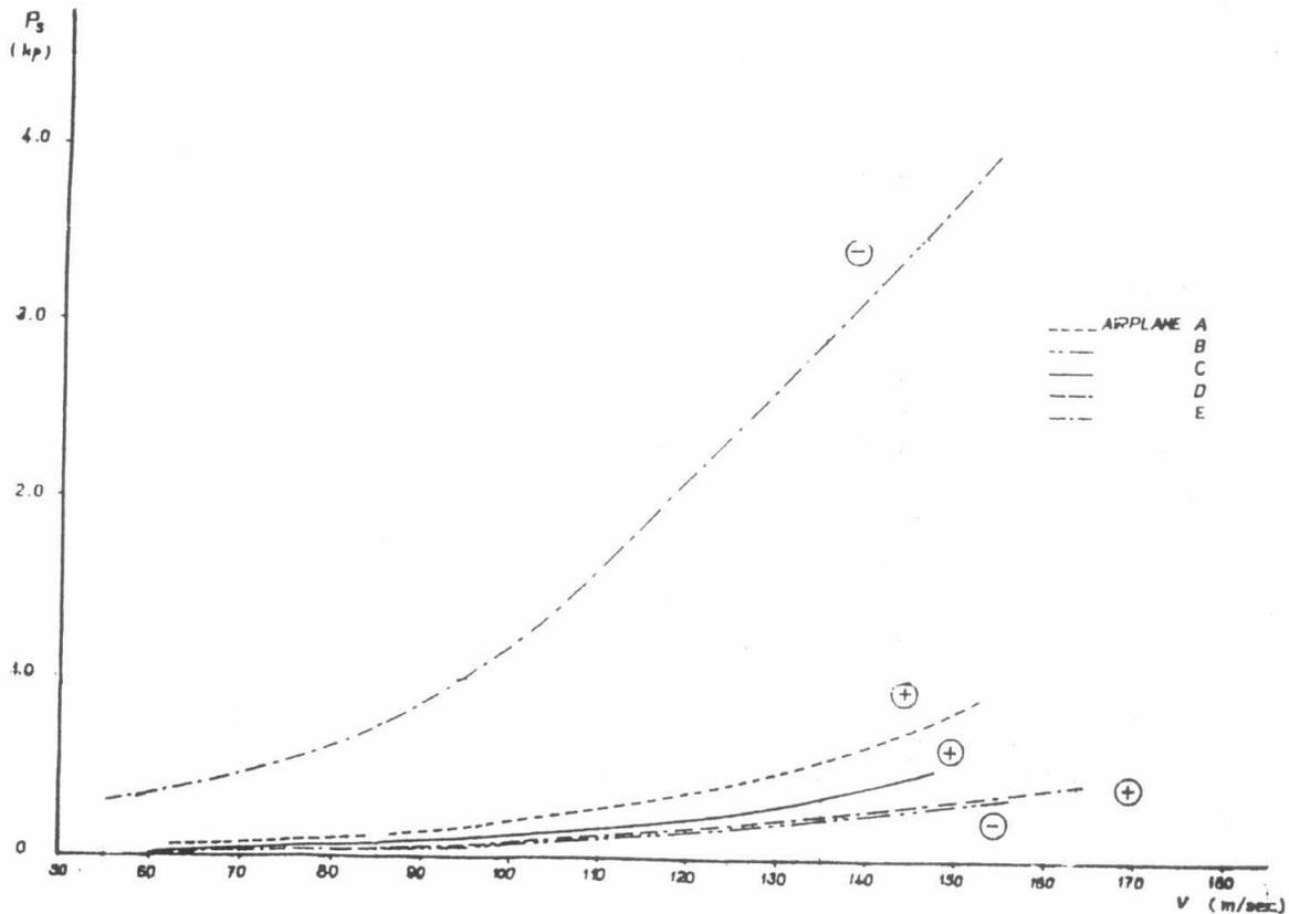
Fig.1, Stick force due to plastic deformation
