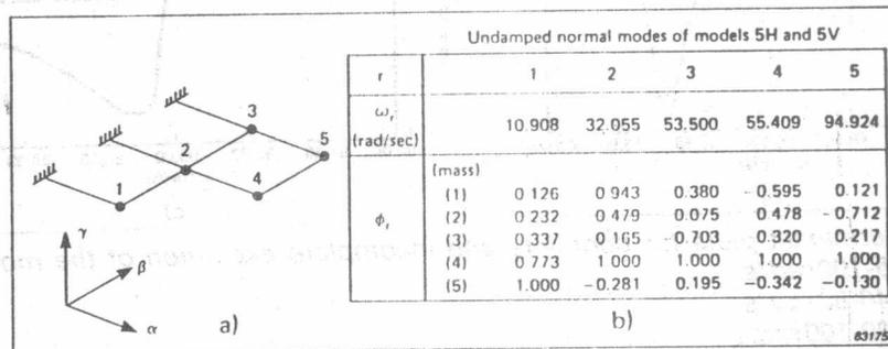
Fig.1 a) Structure of the model
