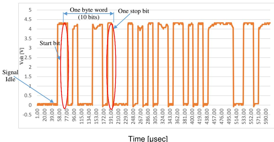
**Fig. 5.** Sample ECU message captured on oscilloscope; the signal idle is 0V, the start bit is 4.25V, the stop bit is 0V and the total byte word length is 10 bits (0010111001) or (binary 00111010 = decimal 58 = ASCII character “:”).
