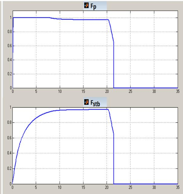
Fig. 27. Sailing system: input response ( $F_p, F_{stb}$  "N" / time "sec")
