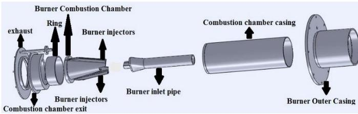
**Figure3: Assembly of EV burner components**
