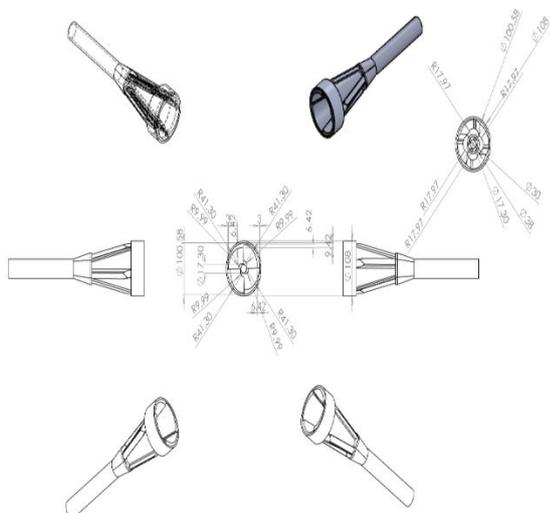
**Figure 5: four slot EV burner.**
