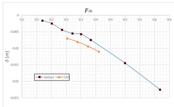
Figure 11. CFD and EFD comparison of sinkage in the Suez Canal
