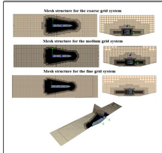
**Figure 10. Mesh structure for the three grid systems in the fluid domain**
