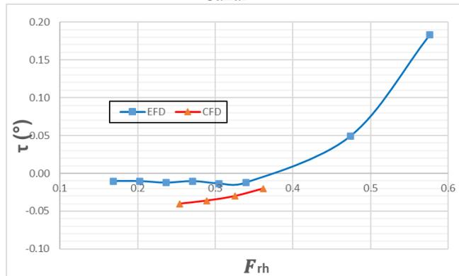
Figure 12. CFD and EFD comparison of trim angle in the Suez Canal
