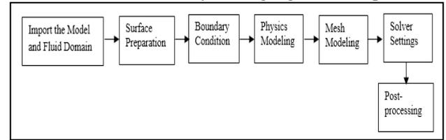
Figure 4. Workflow overview in STAR-CCM+ Source: based on [11]
