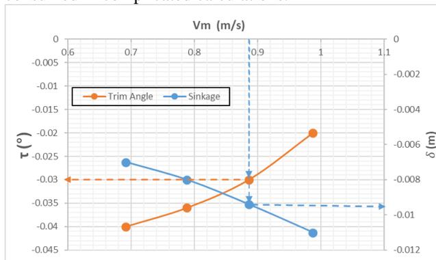
Figure 14. Sinkage and trim angle curves
