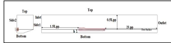
Figure 7. Boundary names of fluid domain
