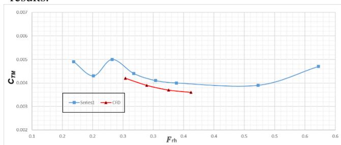
Figure 13. CFD and EFD comparison of total resistance in the Suez Canal
