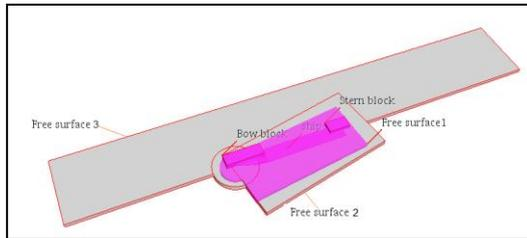
**Figure 9. Multiple blocks for improving mesh resolutions around hull**
