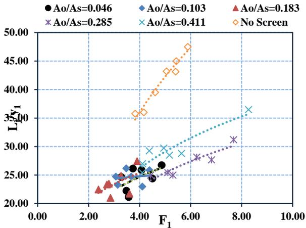
**Figure 9:** Relationship between  $F_1$  and  $L_j/y_1$  for  $S = 3.00$  at different relative holes area of screen fixed at  $l_s/l_a = 0.25$
