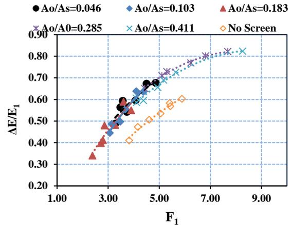
**Figure 5:** Relationship between  $F_1$  and  $\Delta E/E_1$  for  $S = 3.00$  at different relative holes area of screen fixed at  $l_s/l_a = 0.25$
