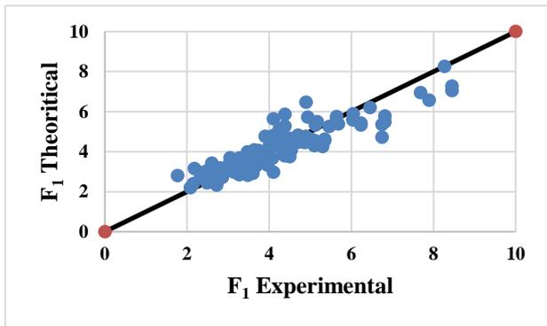
**Figure 13:** Relationship between corrected theoretical  $F_1$  of equation (11) and experimental Froude number
