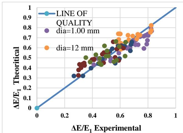
**Figure 14:** Relationship between theoretical  $\Delta E/E_1$  of equation (6) and experimental  $\Delta E/E_1$
