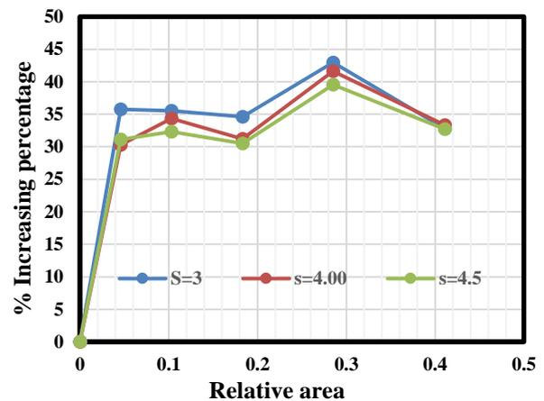
**Figure 6:** Increasing percentage of energy loss for different relative screen holes areas, at  $F_1=4.00$  and  $S=3, 4.0$  and 4.50
