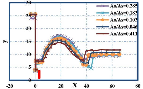
**Figure 11:** Water surface profiles for different relative holes area of screen for  $S = 3.0$ ,  $Q \approx 10.32$ ,  $G = 4.0$
