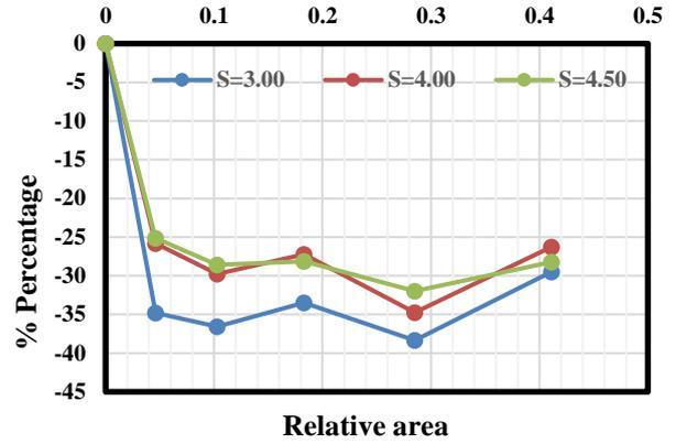
**Figure 10:** Decreasing percentage of relative length of jump for different relative holes area of screen at  $F_1 = 4.50$ ,  $S = 3, 4$  and  $4.50$
