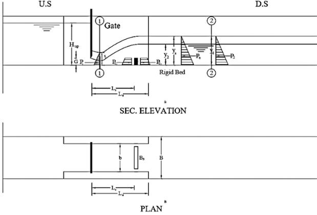
**Figure 4:** Schematic illustration of the submerged hydraulic jump induced by screen
