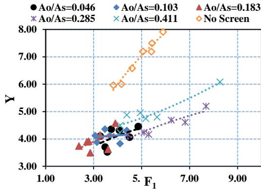
**Figure 7:** Relationship between  $F_1$  and  $Y$  for  $S = 3.00$  at different relative holes area of screen fixed at  $l_s/l_a = 0.25$
