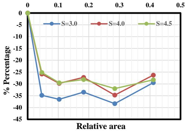
**Figure 8:** Percentage of relative depth of jump for different areas of screen at  $l_s/l_a = 0.25$ ,  $F_1 = 4.50$  and  $S = 3, 4$  and  $4.5$
