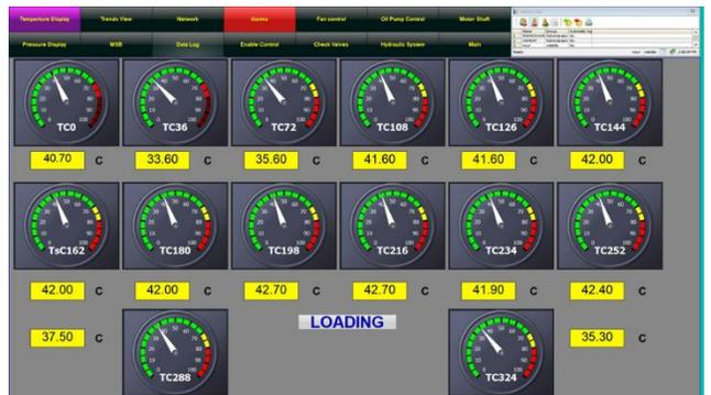
Figure 23: Oil film temperature distribution display page.
