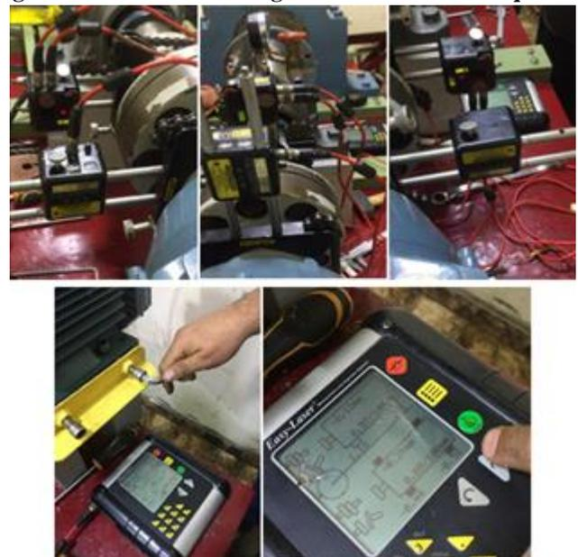
The results were obtained at both horizontal and vertical positions and were also recorded digitally for the UJBTR in the course of the alignment adjustment procedures via the Easy Laser Shaft Alignment System (D525 of Sweden). The following table would represent the results concerning the laser shaft alignment as between the journal shaft and the drive shaft. More important still, those registered values were subject to a continuous update process throughout the alignment adjustment processes.
