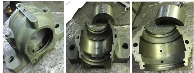
**Figure 8: The modified supporting journal bearing**
