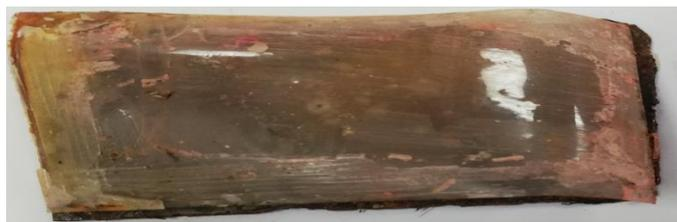
Figure (14): Blank epoxy coated sample after 6 days of HCl exposure
