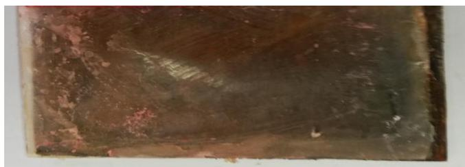
Figure (13): Blank epoxy coated sample after 17 days of NaOH exposure
