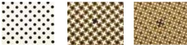
Figure 21: Adaptive fritting system transforms from transparent (left), semitransparent (middle), and opaque status (right) [37]
