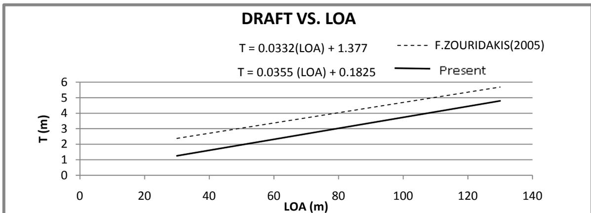
Figure (10): Comparison between ships's T VS. LOA
