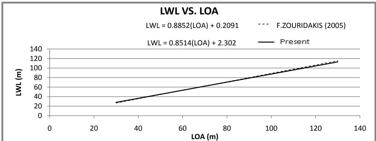
Figure (9): Comparison between ships's LWL VS. LOA
