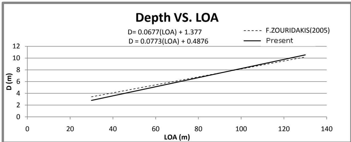
Figure (11): Comparison between ships's D VS. LOA
