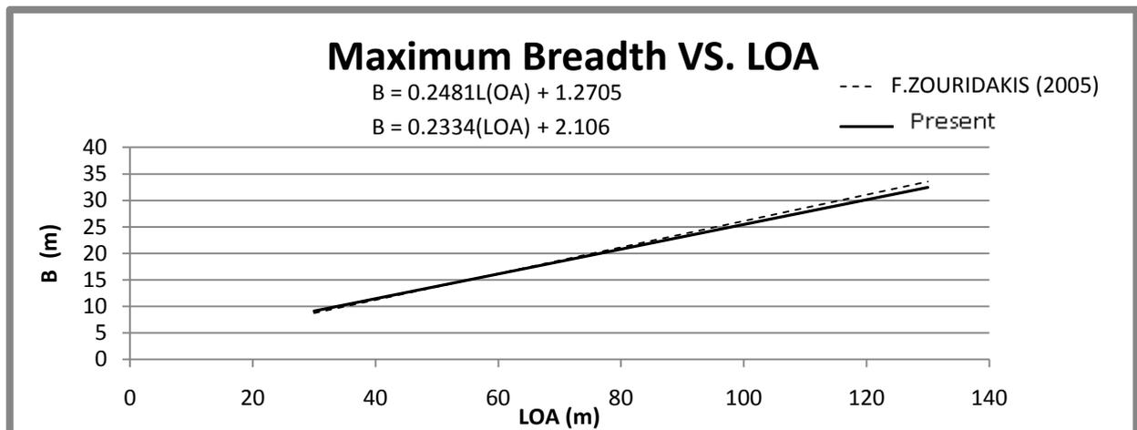
Figure (12): Comparison between ships's B VS. LOA
