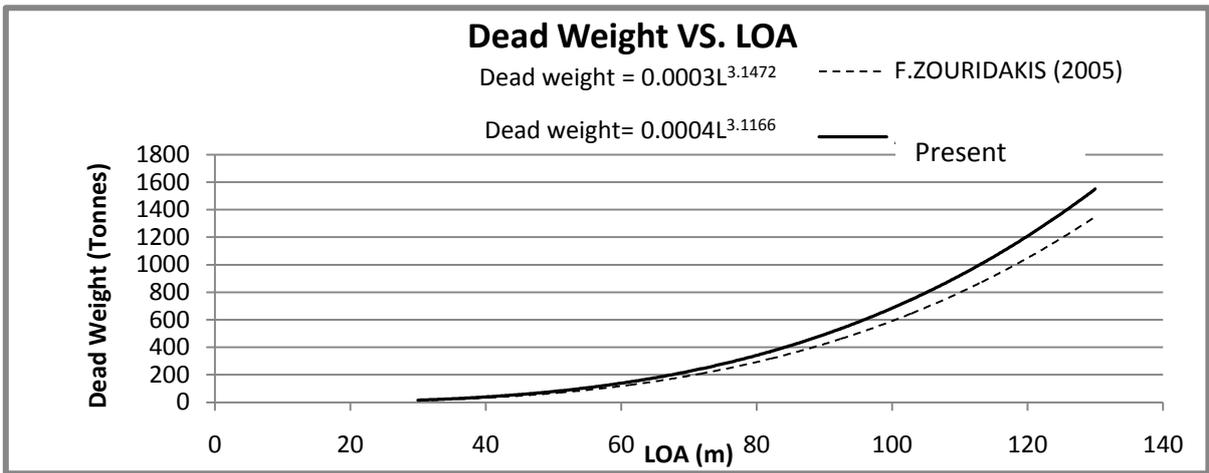
Figure (8): Comparison between ships's DWT VS. LOA
