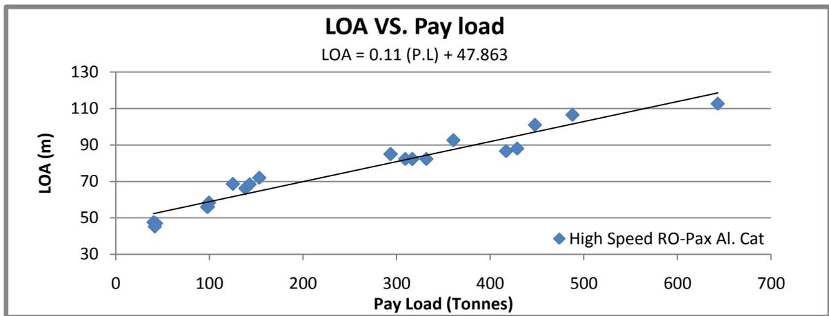
Figure (2): The relationship between LOA VS. Payload
