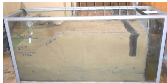
Figure 18: clay wall with depth= 0.75U and distance from canal= 1.875U
