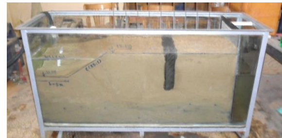
Figure 13: clay wall with depth=0.75U and distance from canal=1.125U
