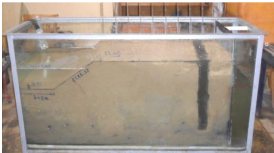
Figure 20: clay wall with depth= 1.5U and distance from canal= 1.875U
