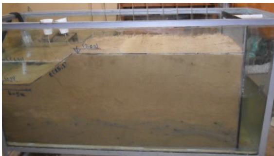
Figure 5': water reaches the highest level at down stream of (h)=50cm, head difference( \Delta H )=15cm .
