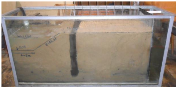
Figure 10: clay wall with depth=1.5U and distance from canal=0.375U
