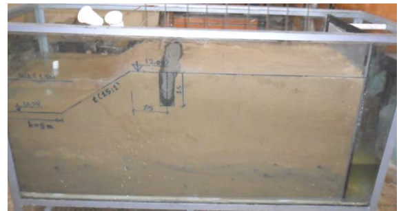
Figure 7: clay wall with depth=0.375U and distance from canal=0.375U
