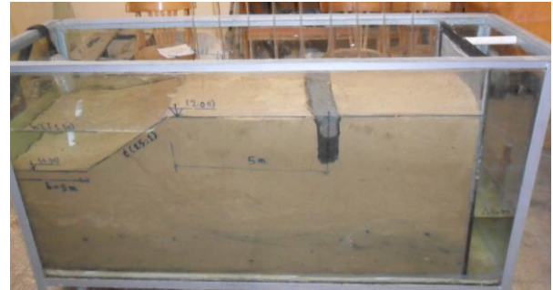
Figure 12: clay wall with depth=0.375U and distance from canal=1.125U
