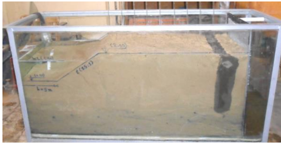
Figure 19: clay wall with depth= 1.125U and distance from canal= 1.875U
