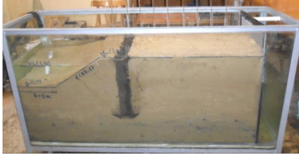
Figure 9: clay wall with depth=1.125U and distance from canal=0.375U
