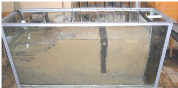
Figure 14: clay wall with depth= 1.125U and distance from canal= 1.125U
