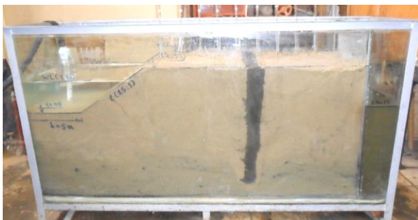
Figure 15: clay wall with depth= 1.5U and distance from canal= 1.125U
