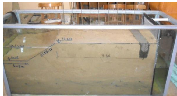
Figure 17: clay wall with depth= 0.375U and distance from canal= 1.875U
