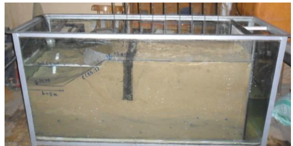
Figure 8: clay wall with depth=0.75U and distance from canal=0.375U
