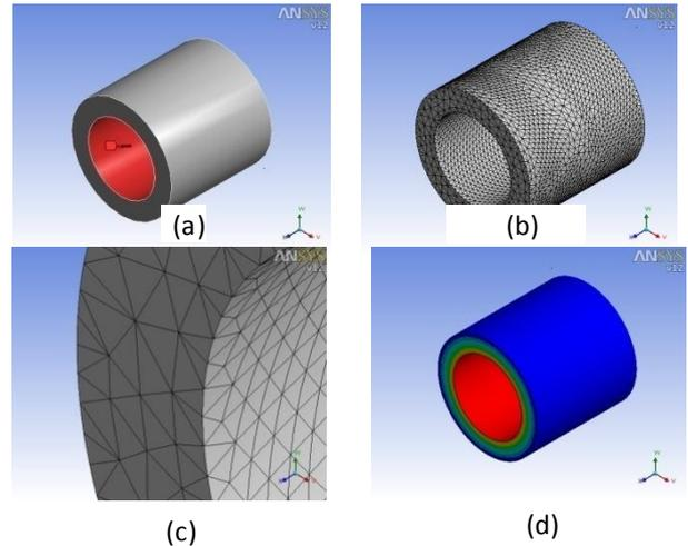
Fig. 3.5: Thick walled cylinder under internal pressure
