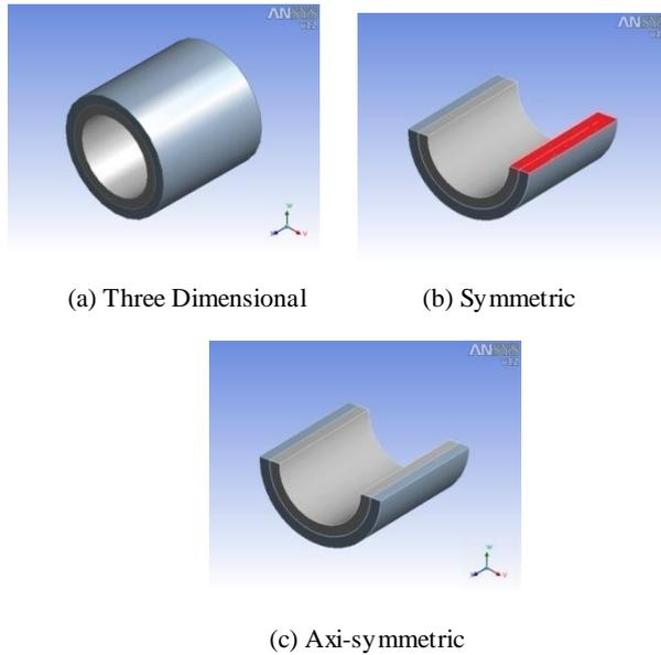
Fig. 3.3: Ways to run the model.
