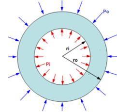
**Fig. 2.1: Thick walled cylinder under**
