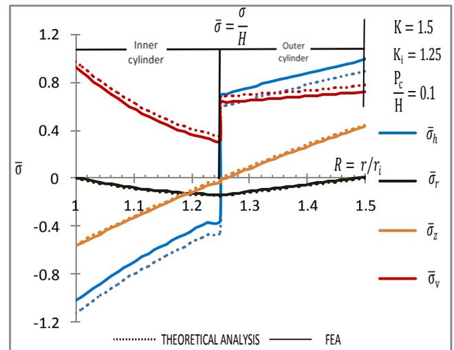
**Fig. 4.5: Stresses distribution for compound cylinder due to constant internal temperature.**
