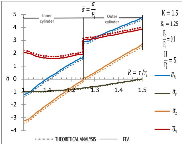
**Fig. 4.6: Stresses distribution for compound cylinder due to constant internal pressure and temperature**
