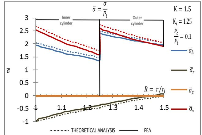
**Fig. 4.4: Stresses distribution for compound cylinder due to constant internal pressure.**
