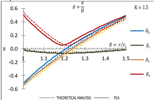
**Fig. 4.2: Stresses distribution on monoblock cylinder due to constant internal temperature.**
