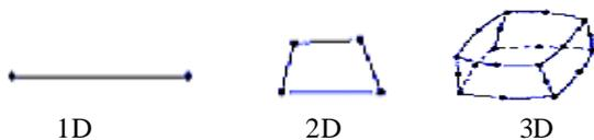
Fig. 3.1: Common element types used in ANSYS simulation.
