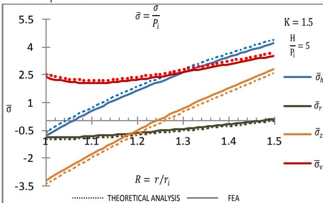
**Fig. 4.3: Stresses distribution on monoblock due to constant internal pressure and temperature.**
