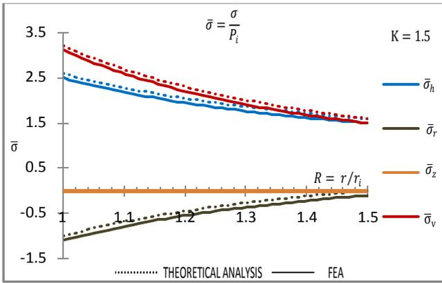
**Fig. 4.1: Stresses distribution on monoblock cylinder due to constant internal pressure.**
