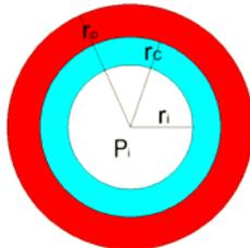
Fig. 2.2: Compound cylinder under
