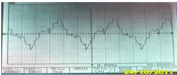
Fig 13: AC voltage measured during hoist up motion
