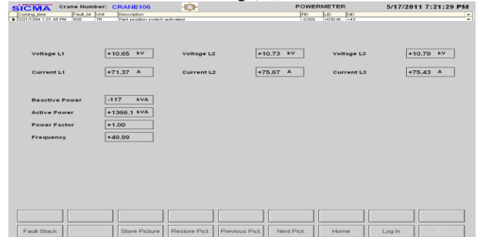
Fig.34: Values from PLC program of the crane
