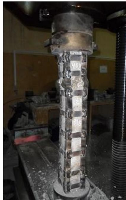
**Fig.11 Jacket failure of group (E)**
