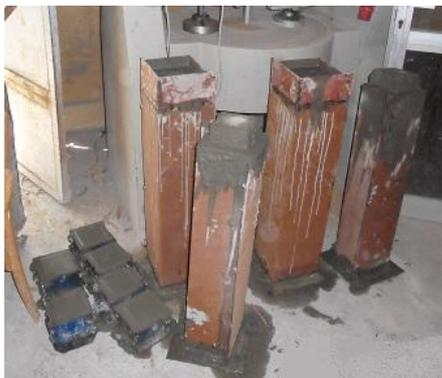
Fig.3 Concrete jacket after casting
