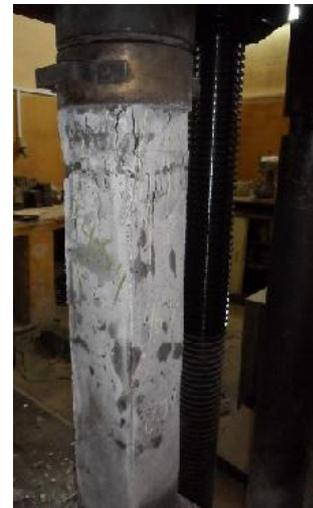
Fig.6 Jacket failure of group (A)
