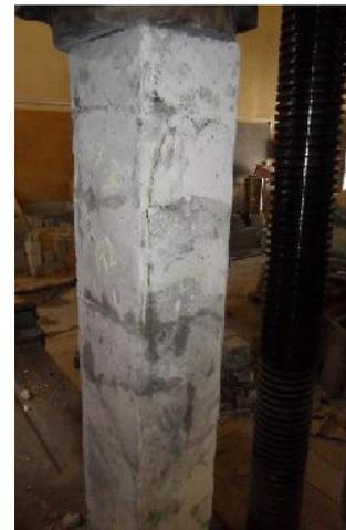
Fig.7 Jacket failure of group (B)
