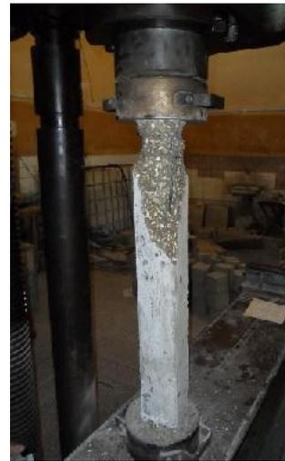
Fig.5 Original column failure
