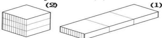
Fig (17) Relationship between Building Surface to its Volume and its effect on gaining and Losing Heat from and to the building. (27)
