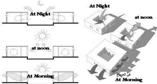
**Fig (11) Difference in direction of Air Movement inside Courtyards during day and night times. (25)**
