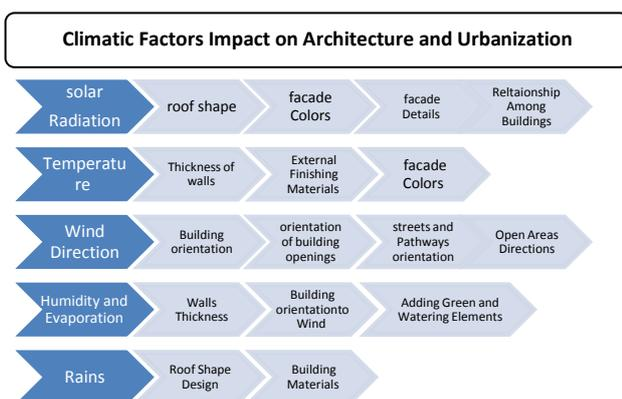
**Fig (4) Effect of Climatic Factors on Architecture** 44
