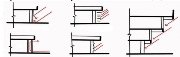
Fig (20) Different Methods to Process External Walls in Hot Areas. (6)
