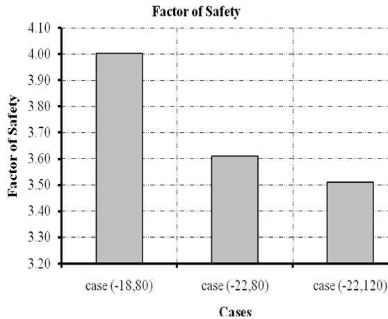
**Figure 18:**  $\phi - c$  reduction factor of safety for three cases.
