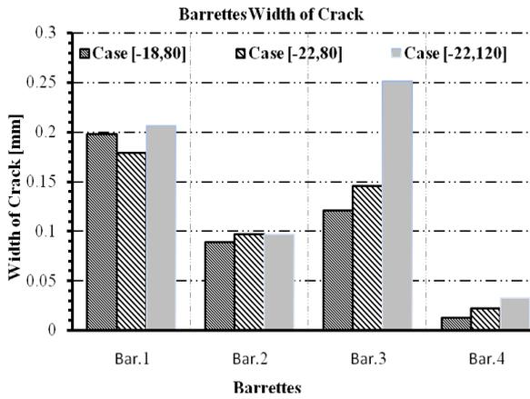
**Figure 13: Width of crack for all barrettes due to the three cases.**
