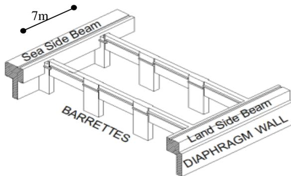
Figure 4: Quay wall beams alignment.
