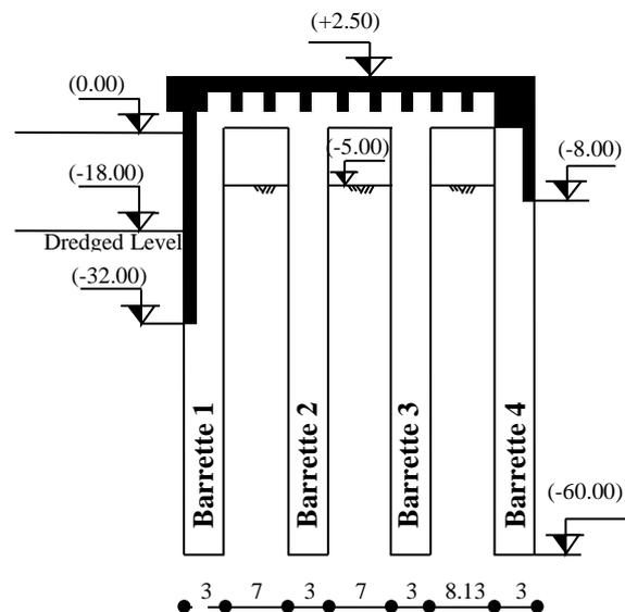
**Figure 3: Quay wall cross section.**
