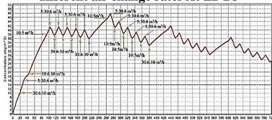
**Figure 37: Predicted TVOC concentrations with different air change rates At Z3-B3**
