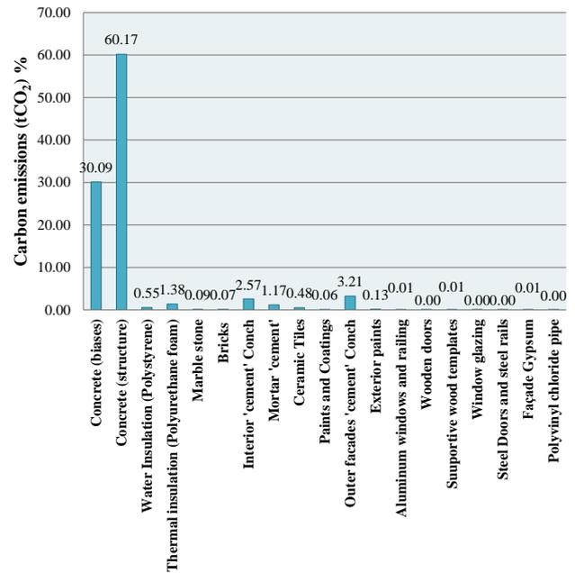
(Figure 3-9) CO<sub>2</sub> emissions resulted from every material type during its transportation phase
