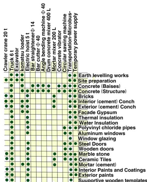
(Figure 3-11) relationship between every material type and machinery used within the process of its construction
