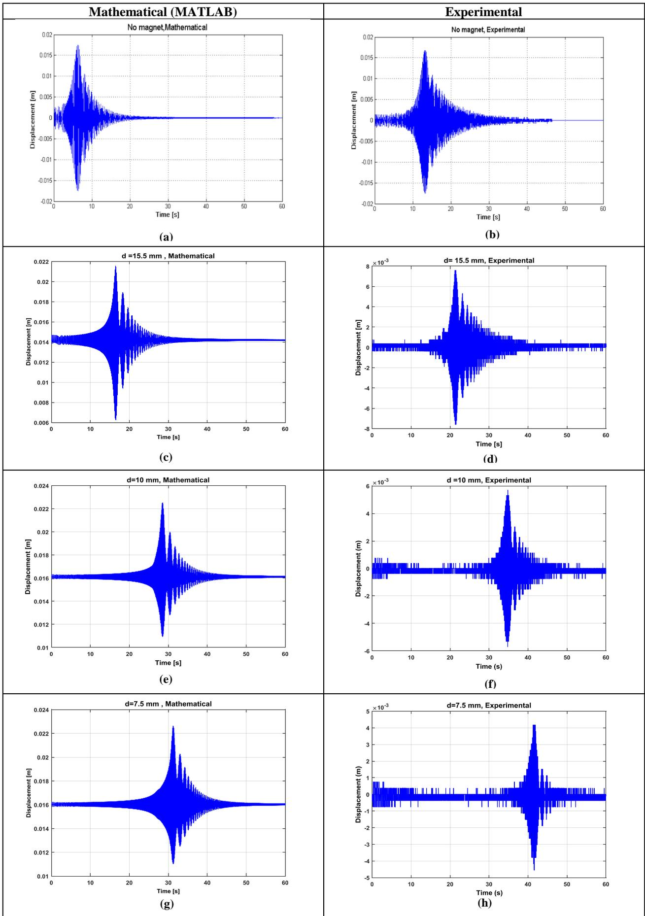
Figure 6 Mathematical and experimental results for the tip displacement of the cantilever beam with frequency sweep from 4 Hz to 20 Hz for different gap distances (a), (b) without magnetic force , (c,d) d=15.5mm, (e,f) d=10mm , (g,h) d=7.5mm
