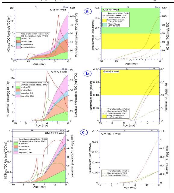
Figure 7 Graphs showing the rates of the generated and expelled oil and gas (left side), in addition to the amounts of expulsion and transformation ratio (right side) for the Lower Rudeis in wells GM-A1(a), GM-G1(b) and GM-4ST1(c).
