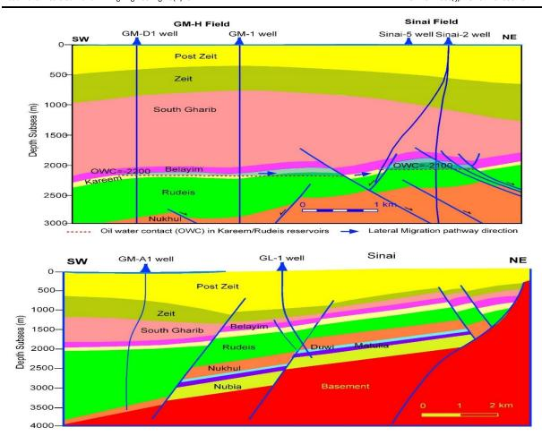
**Figure 9** Geological cross-sections in Garra region indicate the direction of hydrocarbon migration to the northeast direction.
