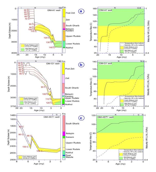
Figure 5 The burial history and maturity models indicate stages of maturity, depth and time to maturity and distribution of temperature of the Lower Rudeis source rock in wells GM-A1 (a), GM-G1 (b) and GM-4ST1 (c).
