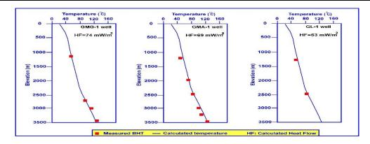
**Figure 4** Plotting of measured temperatures (BHT) and the modelled temperatures shows a good fit for the thermal models.
