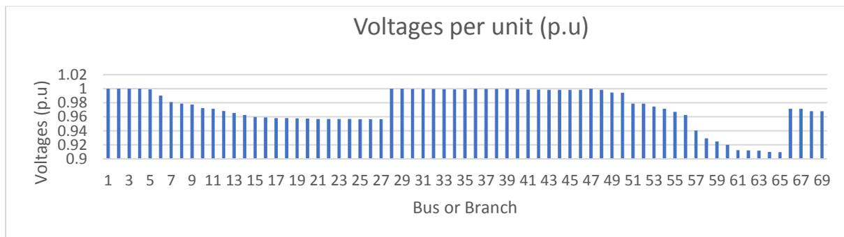
Figure 3 Node Voltage magnitudes of the base case of the IEEE 69-bus
