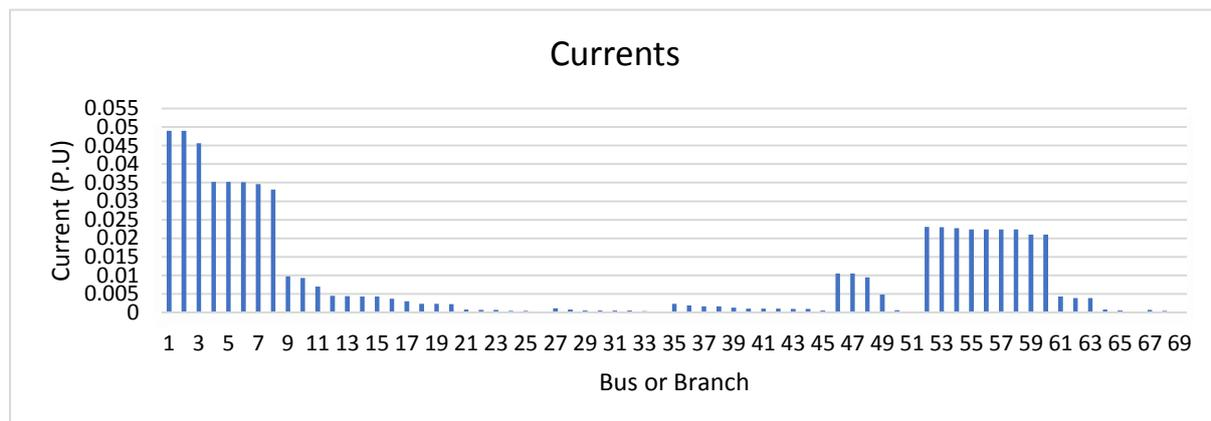
Figure 4 Branch current Magnitude of the base case of the IEEE 69-bus
