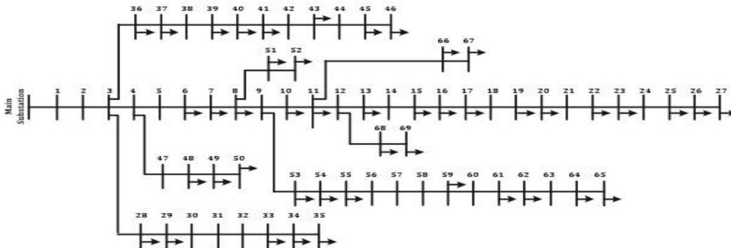
Figure 2 Single line diagram of IEEE 69 bus network
