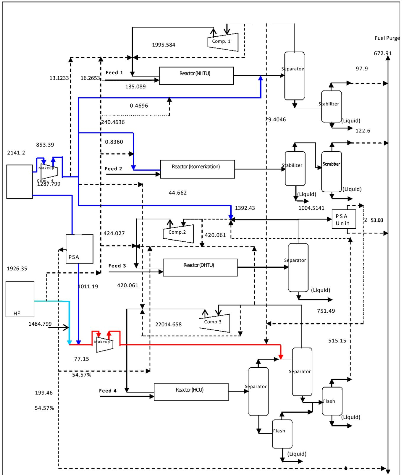
Figure 10. Hydrogen Integration Network with adding a PSA Unit by Cascade Technique.
