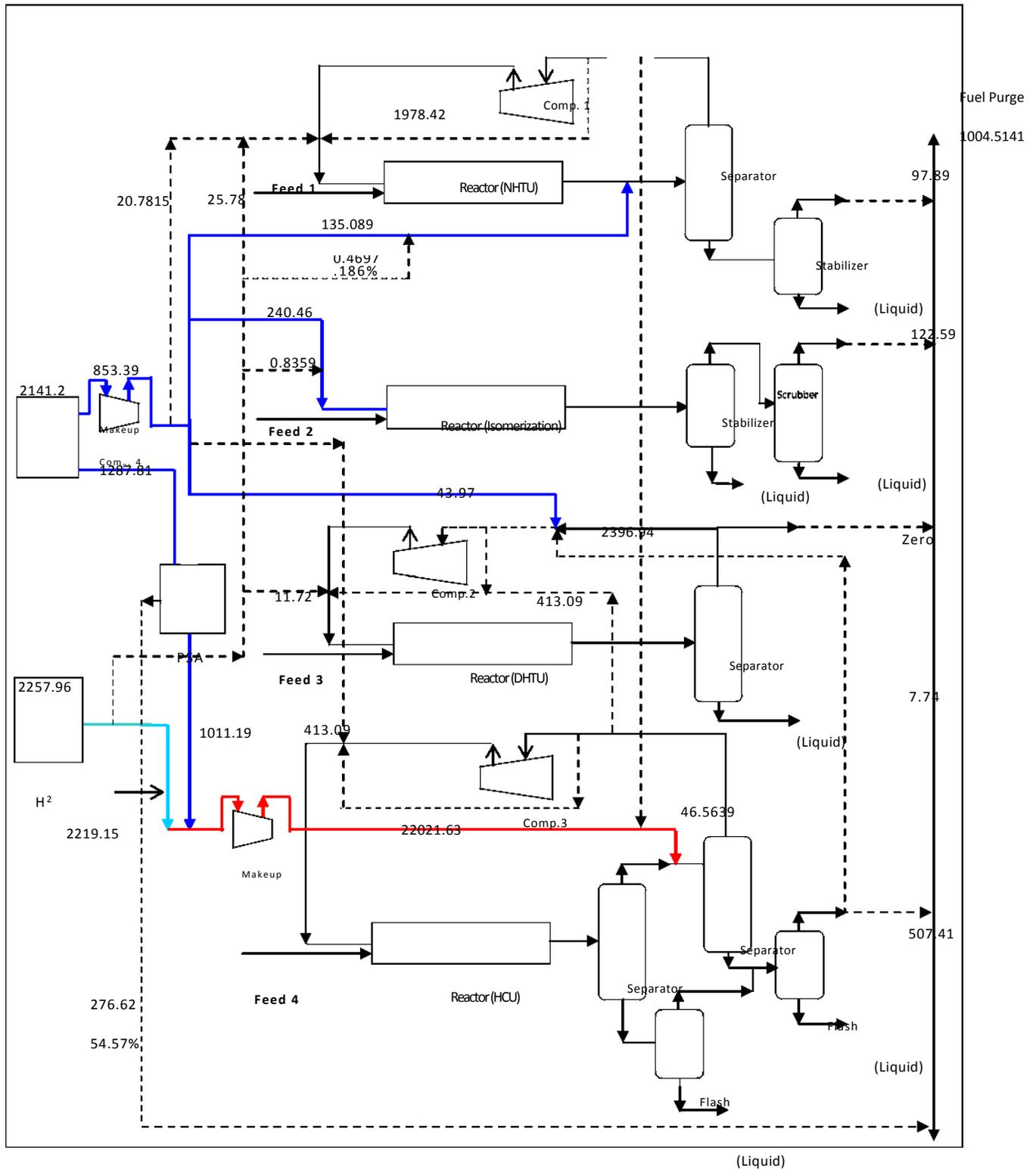
**Figure 8.** Hydrogen Integration Network in the Case Study by Cascade Technique.
