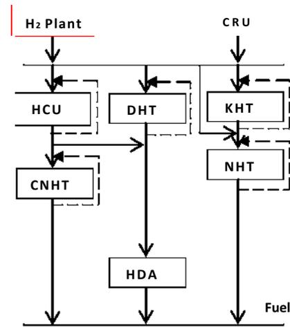
**Figure 1** A typical hydrogen network..
