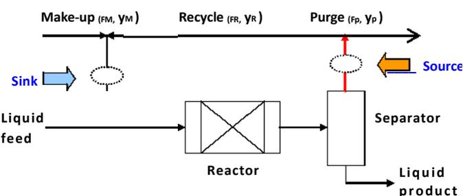
**Figure 2.** Simplified representation of a hydrogen consuming process in hydrogen pinch analysis [13].
