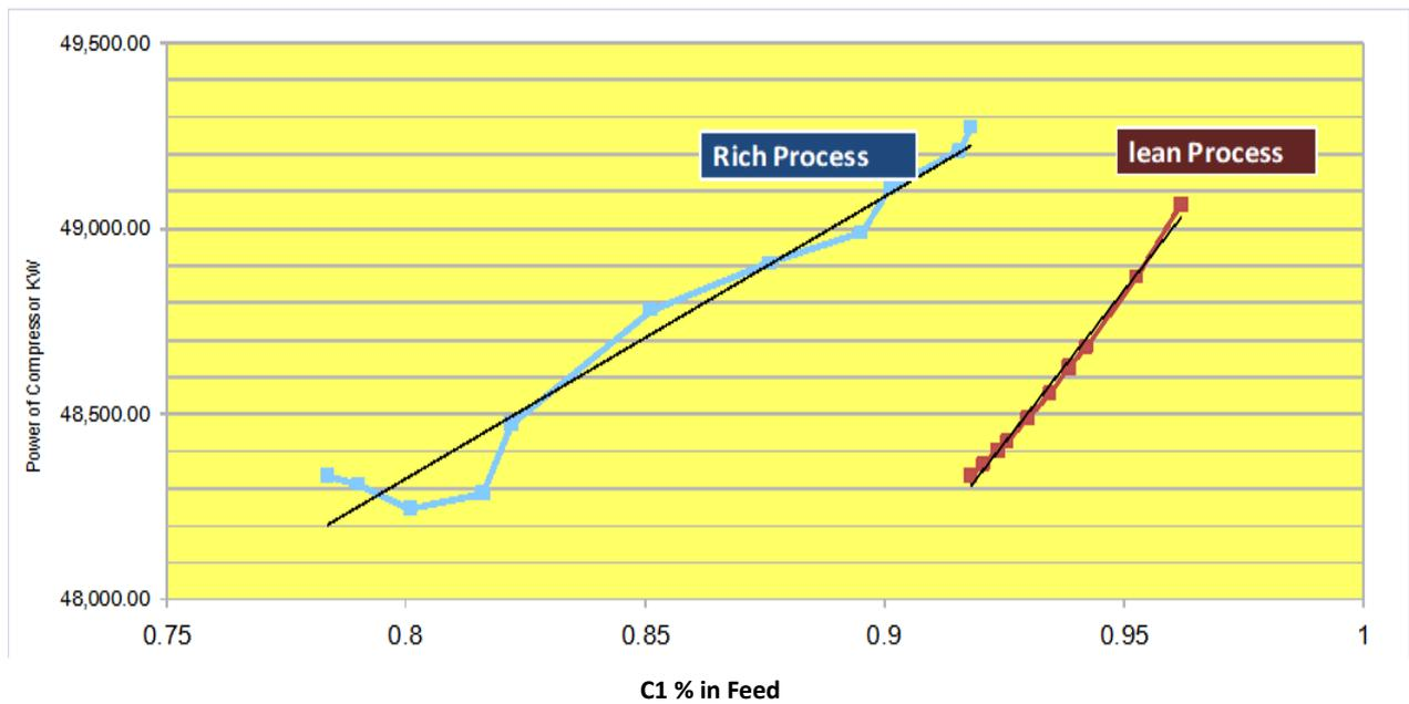
Figure 8 Power of the compressor for Rich and Lean Gas in IOR Process
