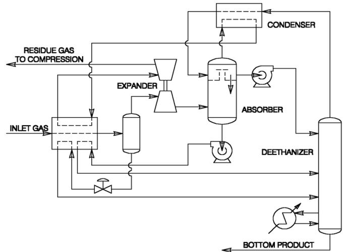
Figure 2 Improved Overhead Recycle process (IOR)
