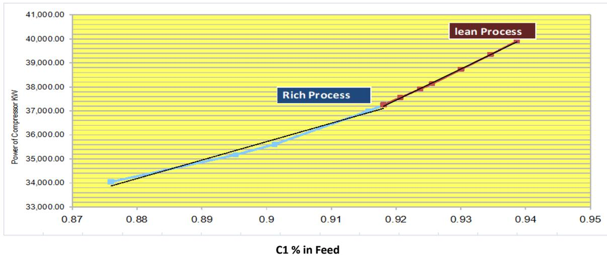
Figure 9 Power of the compressor for Rich and Lean Gas in SCORE Process
