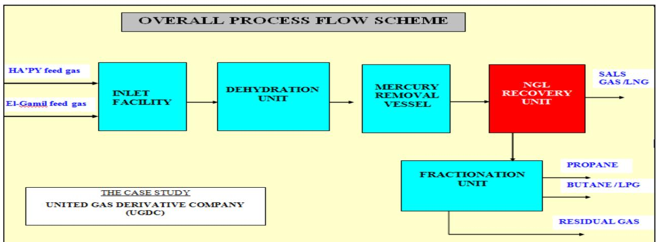
Figure 1 UGDC Overall Process Flow Scheme.
