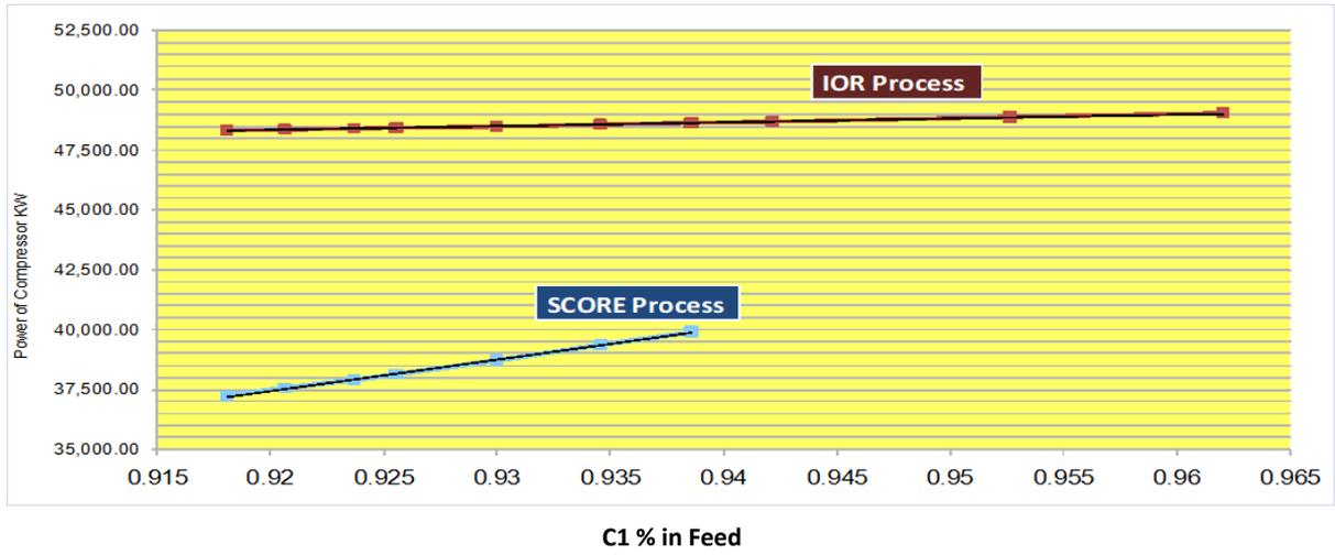
Figure 6 Power of the compressor for Lean Gas in IOR and SCORE Process
