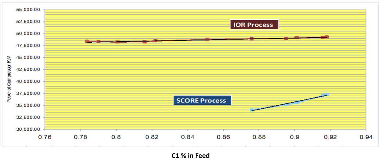
Figure 7 Power of the compressor for Rich Gas in IOR and SCORE Process
