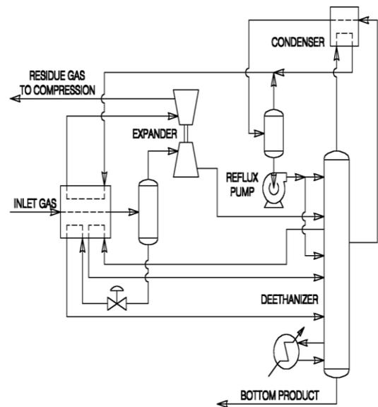
Figure 1 Single Column Overhead Recycle Process (SCORE)
