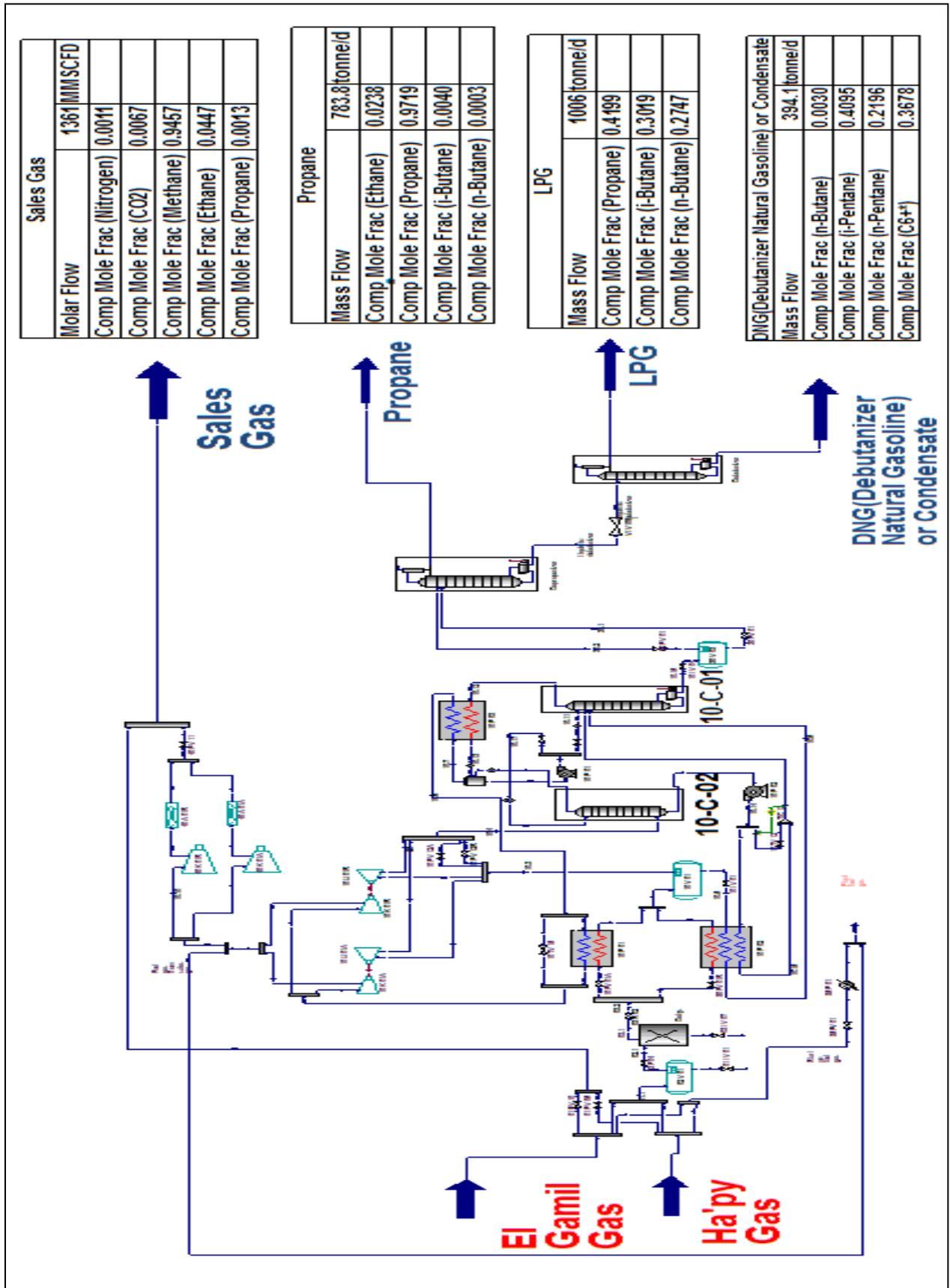
Figure 2 Improved Overhead Recycle Process (IOR)
