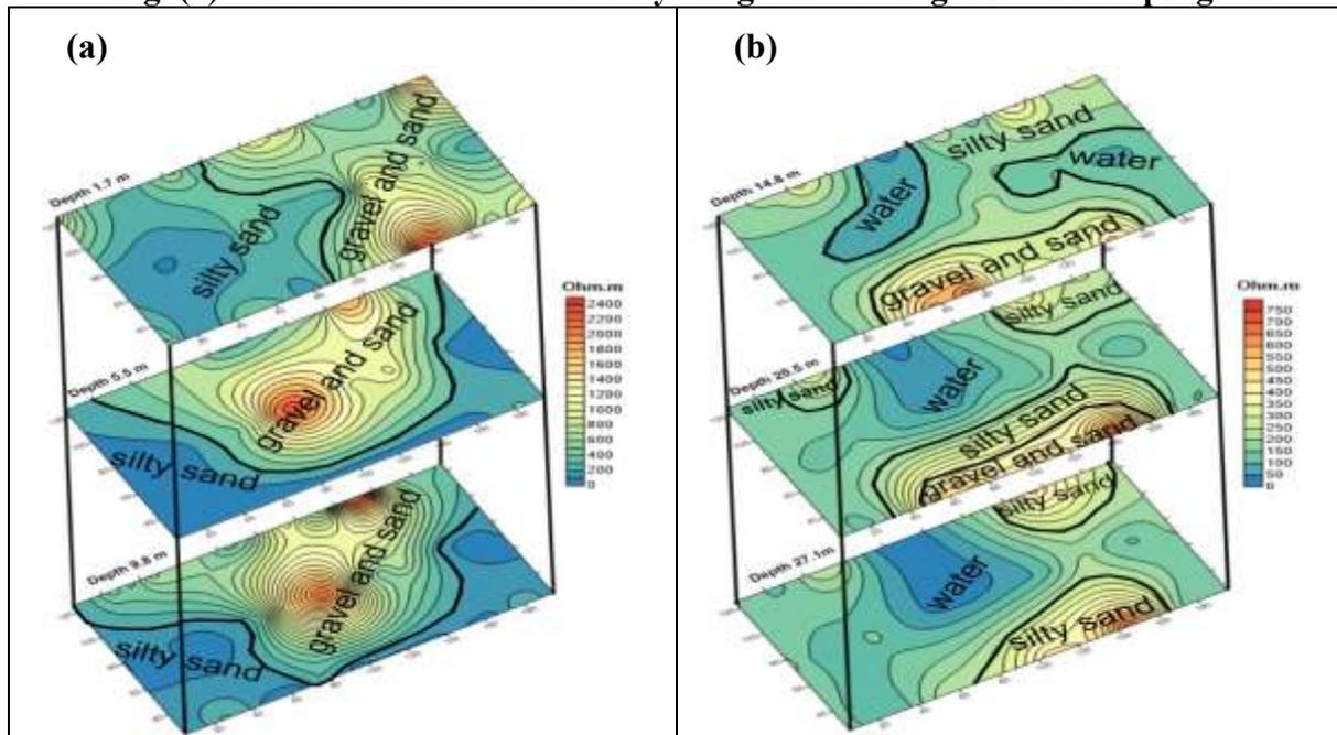
Fig. (7): True Resistivity Map (a) at Depth 1.7 m, 5.5m, 9.8m, and (b) at Depth 14.8m, 20.5m, and 27.1m.
