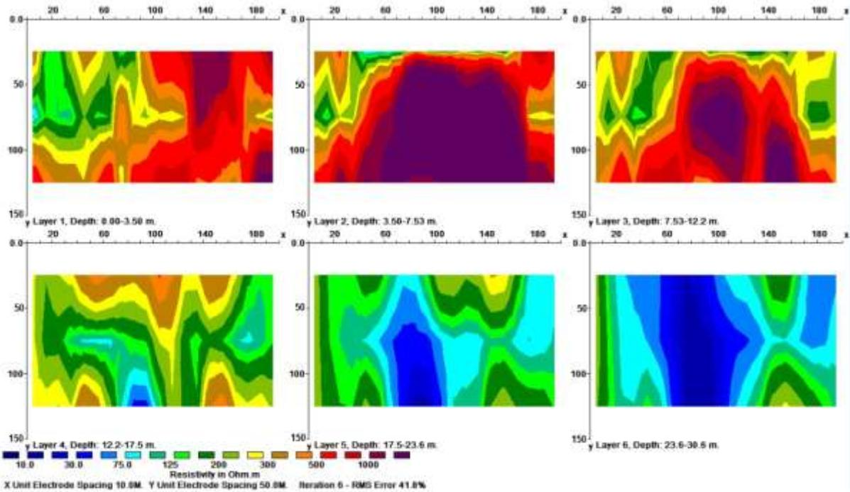
Fig. (6): three-dimensional resistivity image slices using RES3DINV program.
