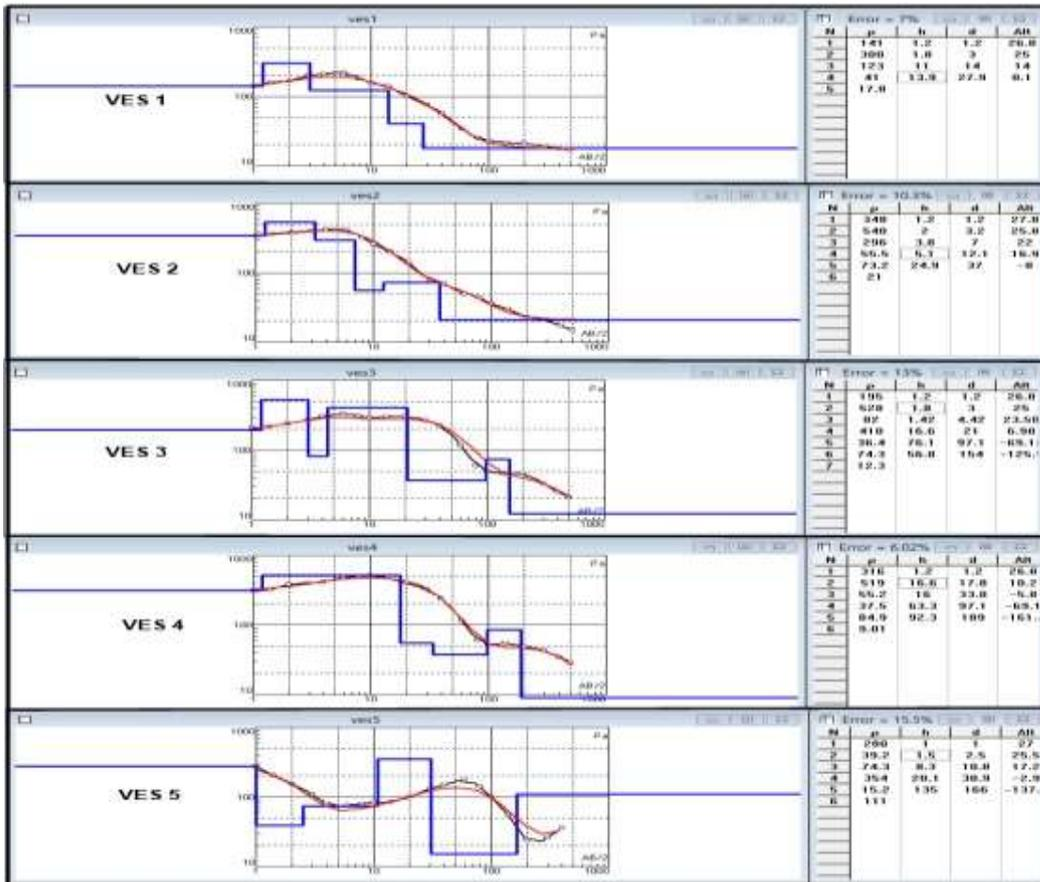
Fig. (3): the resistivity sounding curves for ves 1, ves 2, ves 3, and ves 4 and ves 5.
