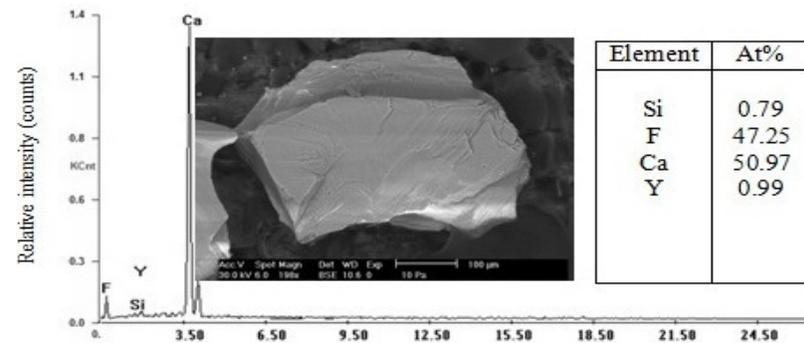
Fig. 20: ESEM spectrograph and BSE image tailed with EDX semiquantitative analysis for violet fluorite separated from El Erediya granitic pegmatites
