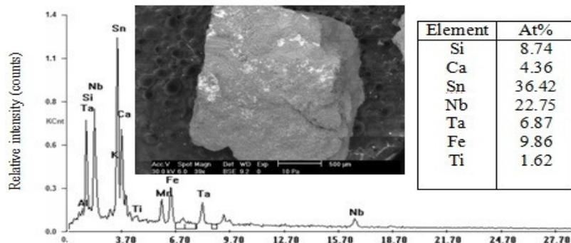
Fig. 19: ESEM spectrograph and BSE image tailed with EDX semiquantitative analysis for cassiterite separated from El Erediya granitic pegmatites.
