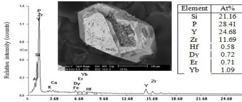
Fig. 18: ESEM spectrograph and BSE image tailed with EDX semiquantitative analysis for xenotime included in El Missikat pegmatitic feldspar
