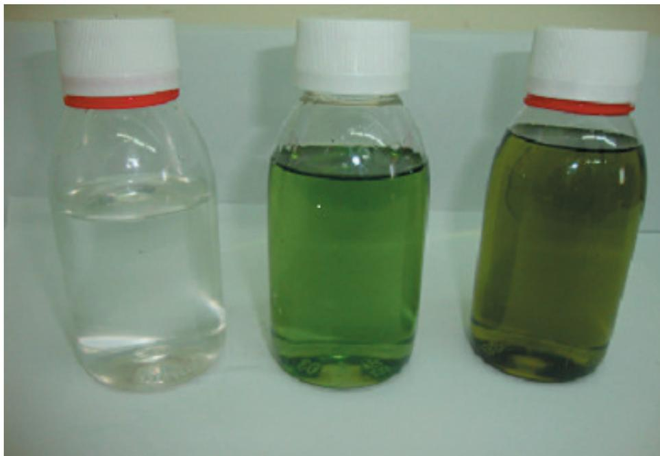
Fig. 18: Comparison between Brown crude phosphoric acid, faint green partially purified phosphoric acid and colorless highly pure grade phosphoric acid
