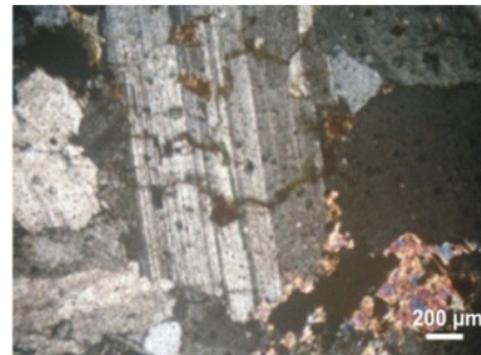
Fig. 12: Photomicrograph showing cracked plagioclase in syenogranite, XPL
