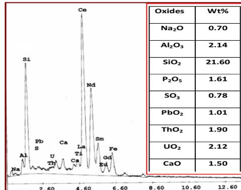
Fig.43: ESEM-EDAX analysis of tornebohmite
