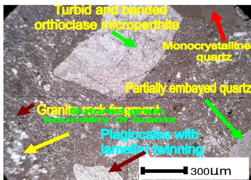
Fig. 14: Photomicrograph shows crystal vitric tuffs and lithic vitric tuffs, XPL
