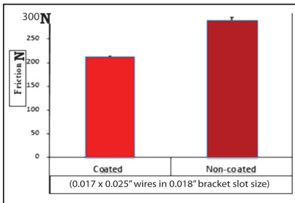
Fig. (4) Effect of coating on friction of 0.017 x 0.025” stainless steel wire in 0.018” ceramic bracket slot size
