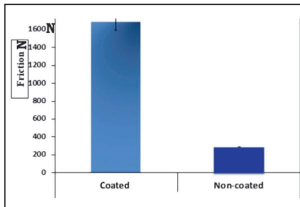
Fig. (5) Bar chart showing the effect of coating on friction of 0.019 x 0.025” stainless-steel wire in 0.022” bracket slot size.
