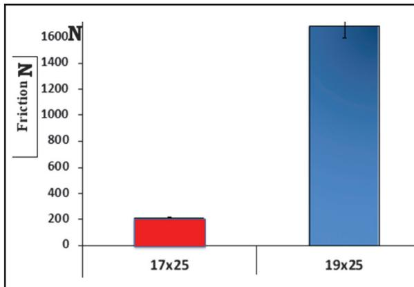
Fig. (6) Effect of coating on friction of coated 0.017 x 0.025” wire in 0.018” bracket slot size and coated 0.019 x 0.025” wire in 0.022” bracket slot size.
