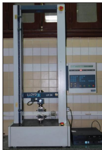
Fig. (2) The LR5K Lloyd universal testing machine.
