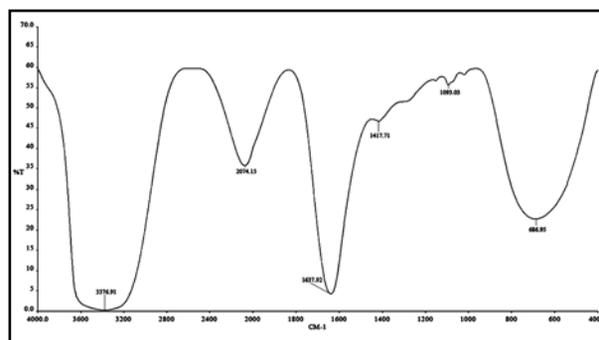
Fig. (1) FTIR spectra of silver nanoparticles stabilized in chitosan by showing their wavelength (cm-1) against their transmittance (%).
