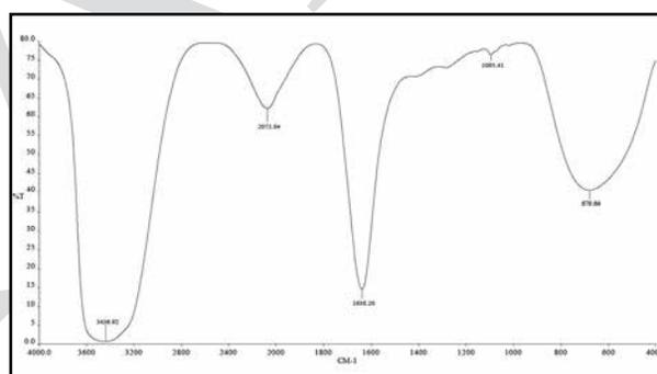
Fig. (2) FTIR spectra of Tetra@ AgNPs by showing their wavelength (cm-1) against their transmittance (%).
