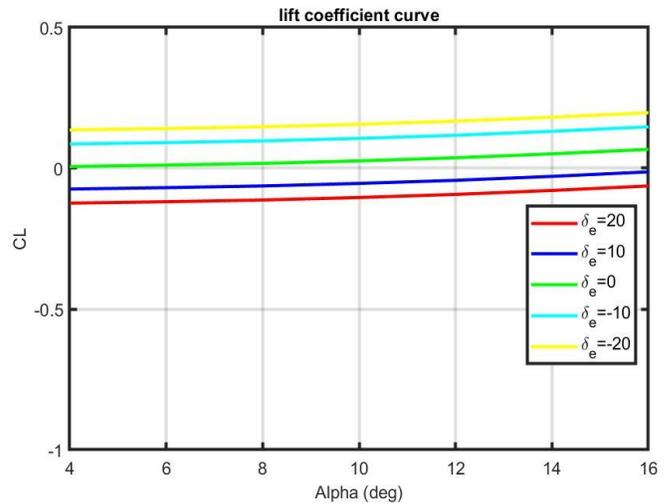
Fig. 9. Lift curve coefficient
