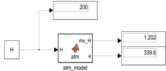
Fig. 6. Simulink atmospheric model
