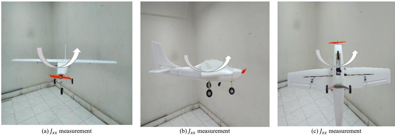
Fig. 2. Moment of inertia measurement setup
