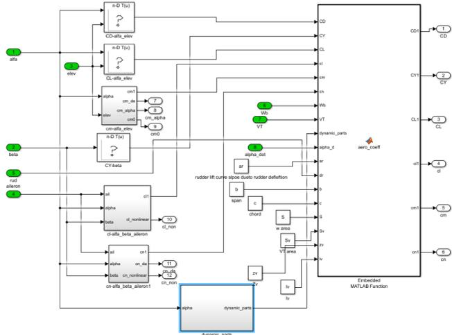
Fig. 5. Simulink aerodynamic model
