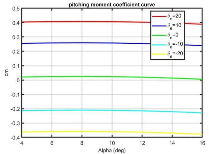
Fig. 10. Pitching moment curve coefficient
