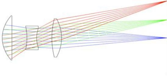
Fig.2. The Cooke Triplet design
