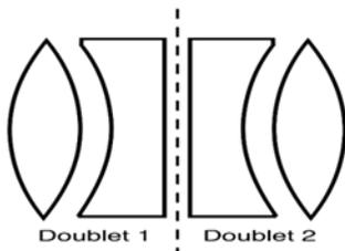
Fig.3 Objective Layout Design
