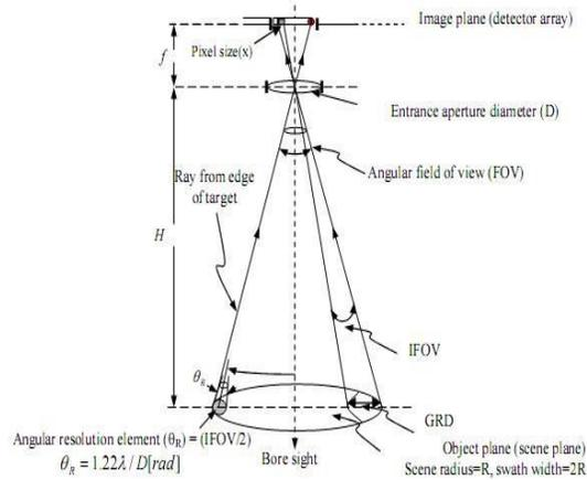
Fig.1 shows optical design parameters of an optical payload
