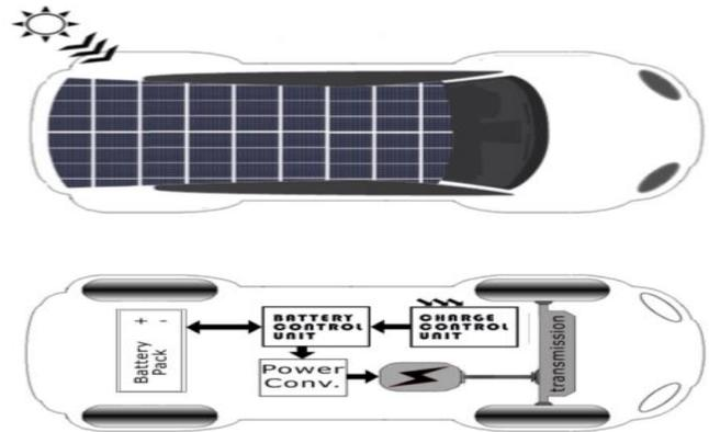
Fig.2 Solar Electric Vehicle drives train with battery pack.
