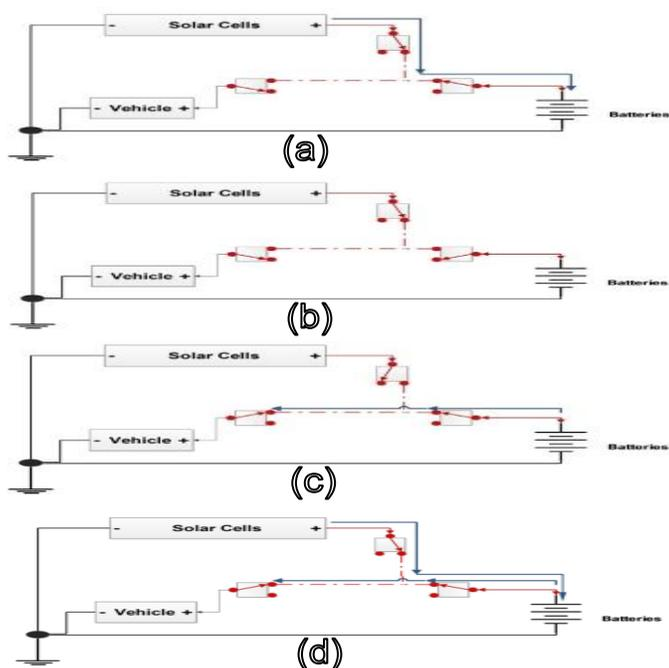
Fig.6 Power management flow diagrams
