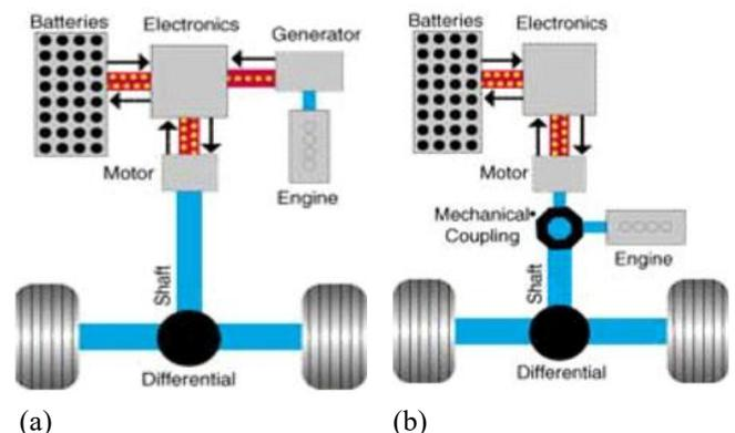
Fig.1 types of hybrid electric vehicles according to way of connection (a) series, (b) parallel.
