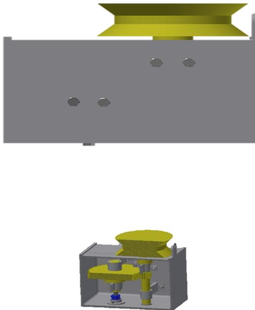
Figure 2.6 turning radius measuring mechanism and cross section of it.
