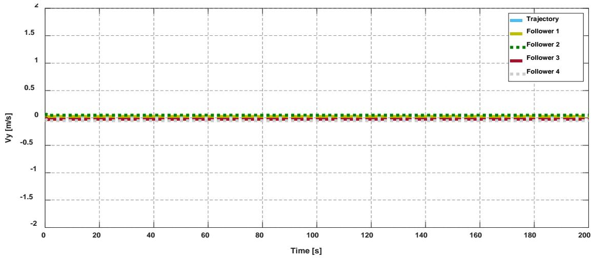
Figure 17. Velocity of cooperative quadrotors in Y-orientation.
