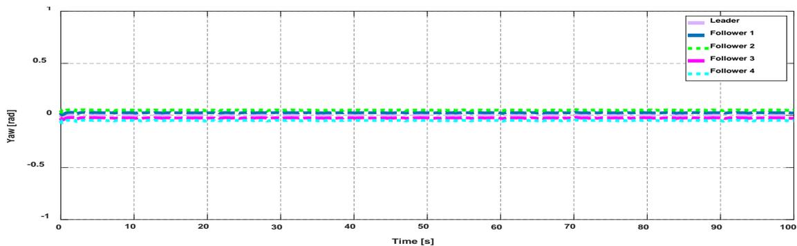
**Figure 13.** Yaw control of BS-PID controller tuned by LOPID for cooperative quadrotors.
