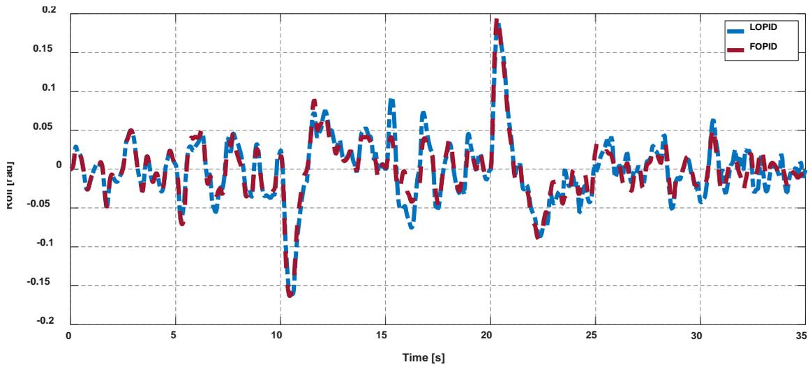
Figure 30. Roll control for BS-PID controller tuned by LOPID and FOPID under effect of noise.
