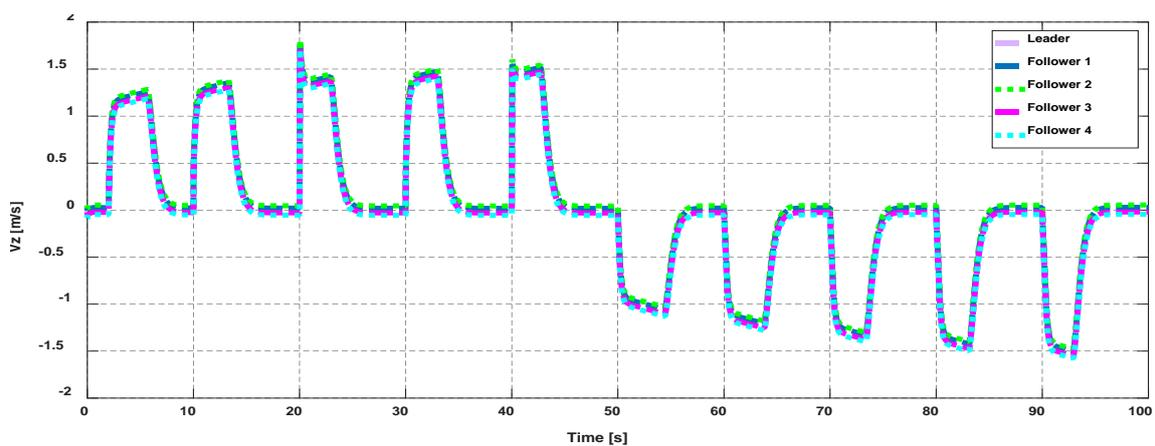
**Figure 8.** Velocity of cooperative quadrotors in *Z*-orientation.
