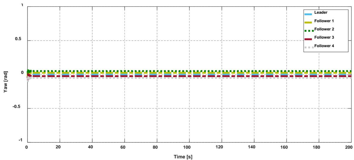
**Figure 24.** Yaw control of BS-PID controller tuned by FOPID for cooperative quadrotors.
