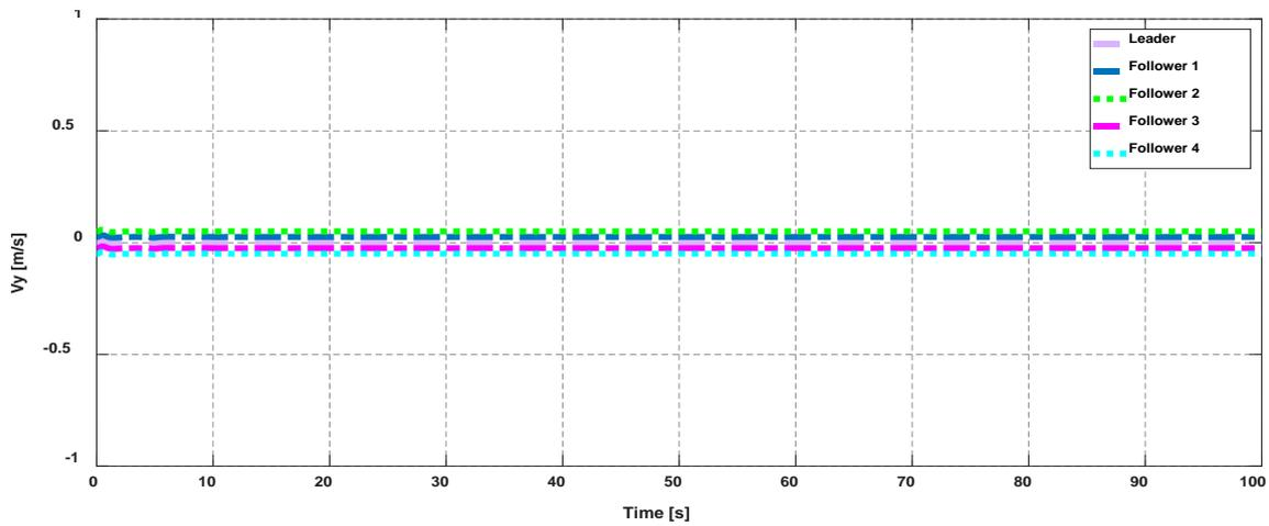
**Figure 6.** Velocity of cooperative quadrotors in *Y*-orientation.
