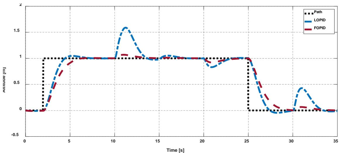
Figure 25. Trajectory tracking of BS-PID controller tuned by LOPID and FOPID for the leader of the cooperative quadrotors in Z-orientation under effect of wind disturbance.
