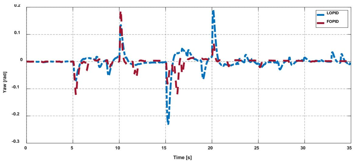
Figure 32. Yaw control for BS-PID controller tuned by LOPID and FOPID under effect of noise.
