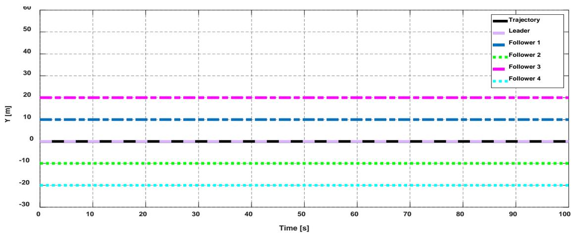
Figure 5. Trajectory tracking of BS-PID controller tuned by LOPID for cooperative quadrotors in Y-orientation.
