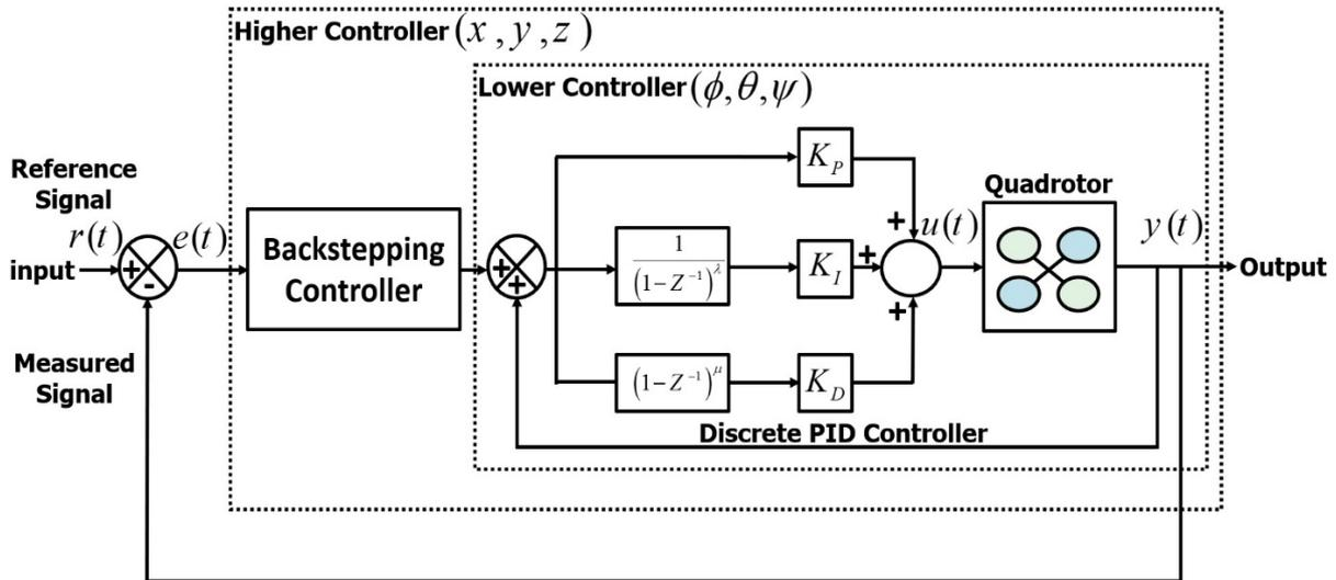
Figure 2. FOPID block diagram for 2<sup>nd</sup> order model of quadrotor framework.
