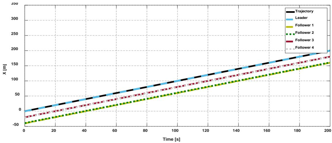
**Figure 14.** Trajectory tracking of BS-PID controller tuned by FOPID for cooperative quadrotors in X-orientation.
