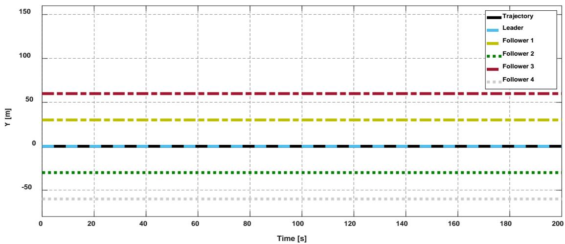
**Figure 16.** Trajectory tracking of BS-PID controller tuned by FOPID for cooperative quadrotors in Y-orientation.
