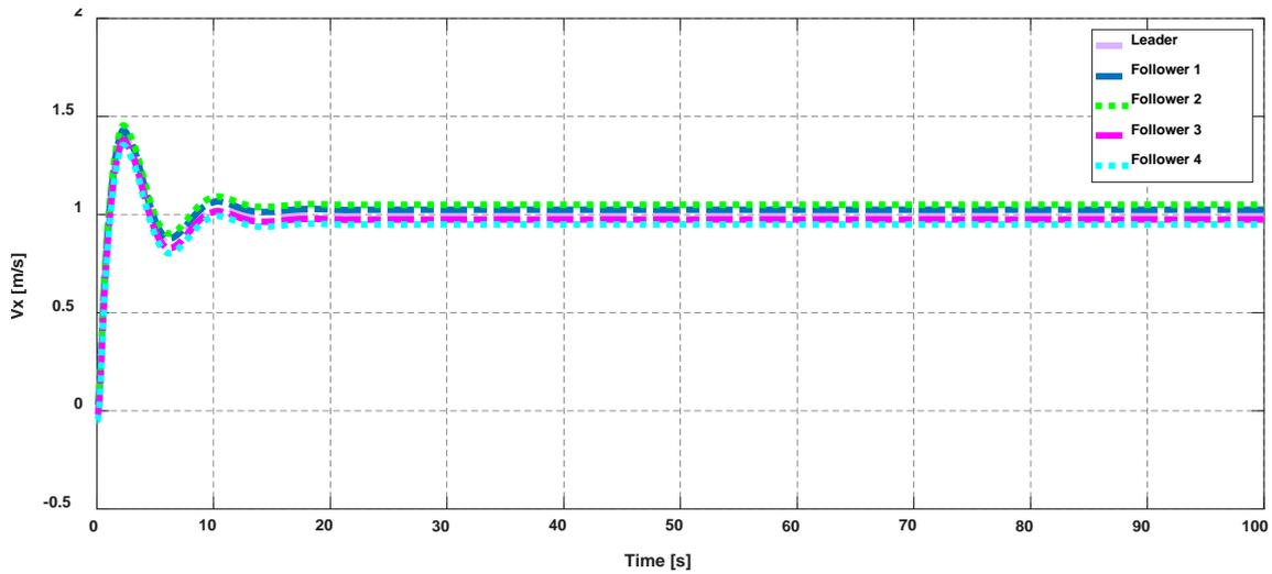
Figure 4. Velocity of cooperative quadrotors in X-orientation.
