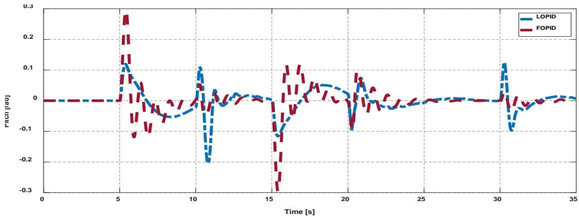
**Figure 27.** Pitch control for BS-PID controller tuned by LOPID and FOPID under effect of wind disturbance.
