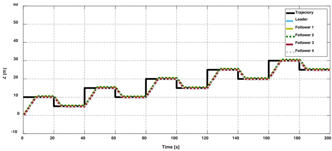
Figure 18. Trajectory tracking of BS-PID controller tuned by FOPID for cooperative quadrotors in Z-orientation.
