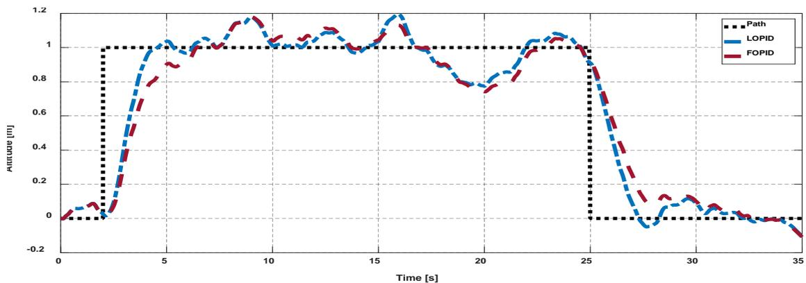
**Figure 29.** Trajectory tracking of BS-PID controller tuned by LOPID and FOPID for the leader of the cooperative quadrotors in Z-orientation under effect of noise.
