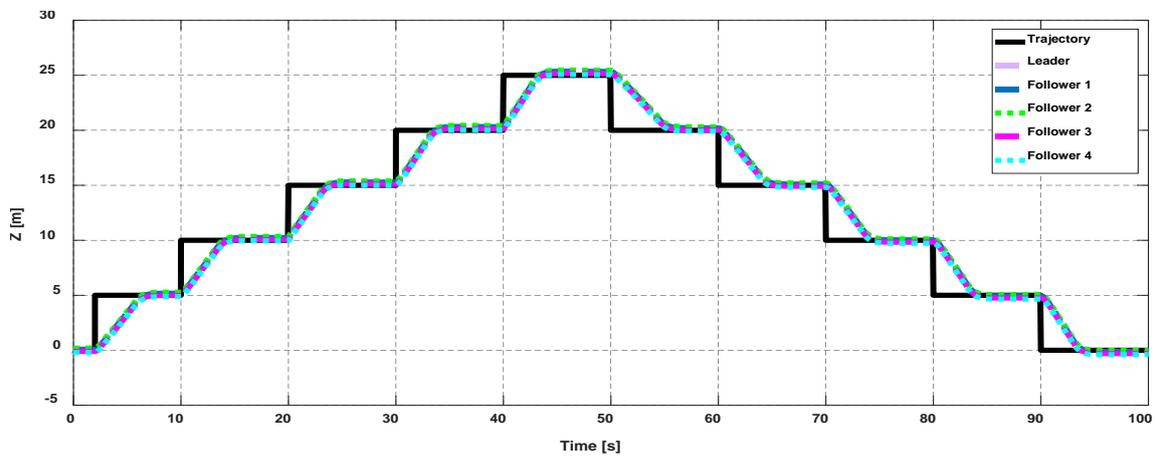
**Figure 7.** Trajectory tracking of BS-PID controller tuned by LOPID for cooperative quadrotors in *Z*-orientation.
