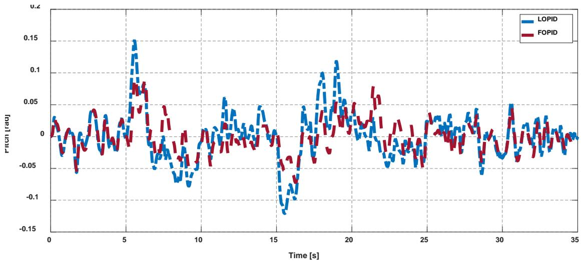
Figure 31. Pitch control for BS-PID controller tuned by LOPID and FOPID under effect of noise.
