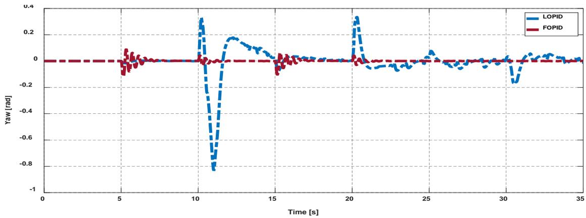
**Figure 28.** Yaw control for BS-PID controller tuned by LOPID and FOPID under effect of wind disturbance.
