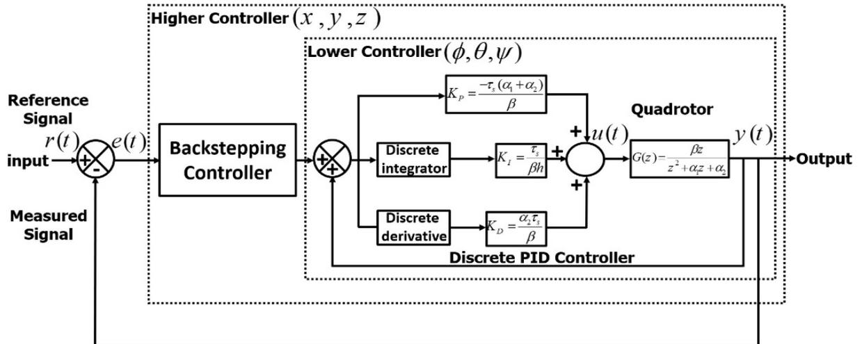
Figure 1. LOPID block diagram for 2<sup>nd</sup> order model of quadrotor framework.
