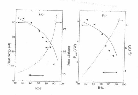
Fig. 4. Variation of (a) output pulse energy and pulse width (b) average and peak powers as functions of output coupler reflectivity at  $T_0 = 80\%$ . The symbols represent the experimental results of Liu et al. [11].
