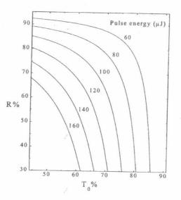
Fig. 5. Plots for some defined values of output pulse energies yielded from various combinations between  $T_0$  and R.
