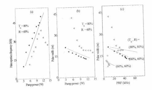
Fig. 6. Dependencies of (a) the pulse width and (b) pulse repetition frequency on the pump power for  $T_0$ =80% and R=60%. The symbols are the experimental data of Liu et al. [11] (empty symbols) and Ng et al. [12] (solid symbols). (c) Variation of the pulse width against the pulse repetition frequency for: i) $T_0$ =80%, R=80% ii)  $T_0$ =80%, R=60% and compared to the experimental ones of [11] iii) T0=60% and R=60% and compared to the experimental ones of [12].
