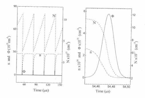
**Fig. 2.** Numerical simulation of passively Q-switching rate equations. (a) General view and (b) details of temporal profiles for Nd:GdVO<sub>4</sub> laser population inversion "*N*", Cr<sup>4+</sup>:YAG ground state population "*n*" and cavity photon density " $\Phi$ " at T<sub>0</sub> = 80% and R = 80%.
