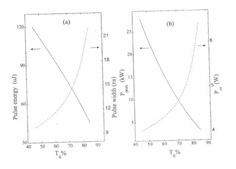
Fig. 3. Dependence of the Q-switched laser parameters: (a) output pulse energy and pulse width (FWHM) (b) Average and peak powers, on the initial transmission of  $Cr^{4+}$ :YAG at R = 80%.
