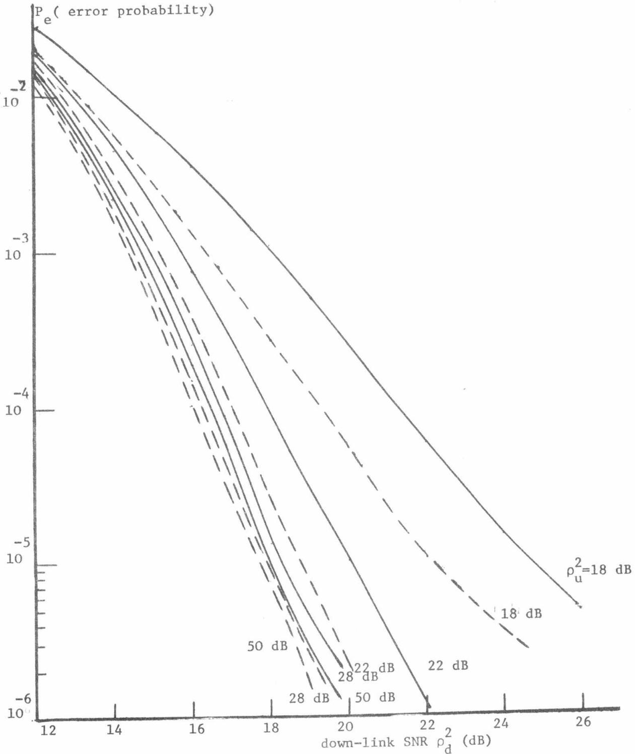
Fig.3. Symbol error probability of 16-ary offset QAM single transmission for various values of up-link SNR  $\rho_u^2$  and back-off levels :-
