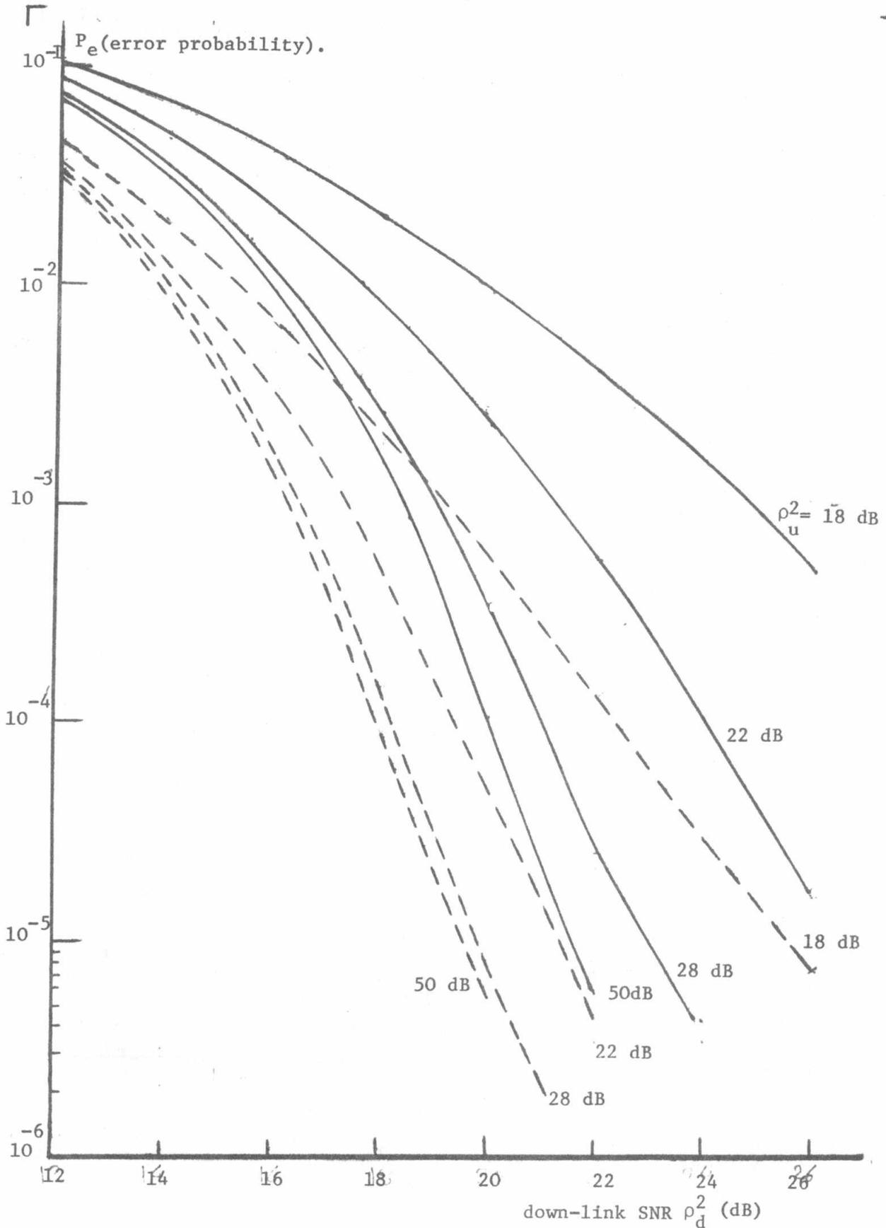
Fig.2. Symbol error probability of 16-ary offset QAM signal transmission for various values of up-link SNR  $\rho_u^2$  and back-off levels
