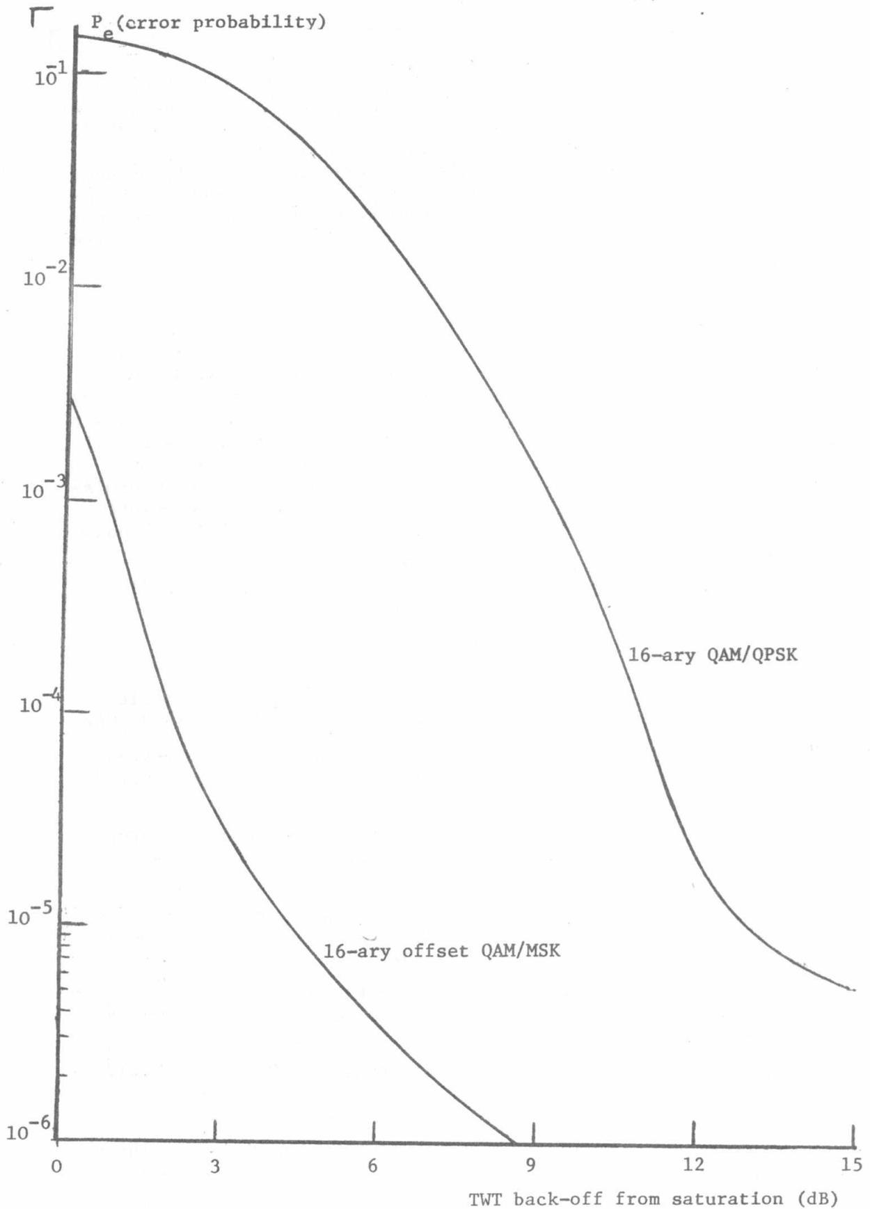
Fig.4. Error probability as a function of TWT back-off from saturation for 16-ary offset QAM/MSK and 16-ary QAM/QPSK transmission with  $\rho_u^2 = 28$  dB and  $\rho_d^2 = 22$  dB
