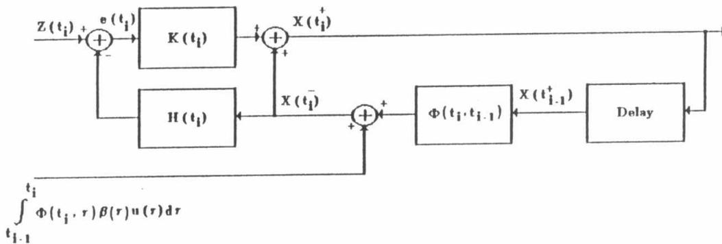
Fig.(2) A Schematic Diagram of the Estimator
