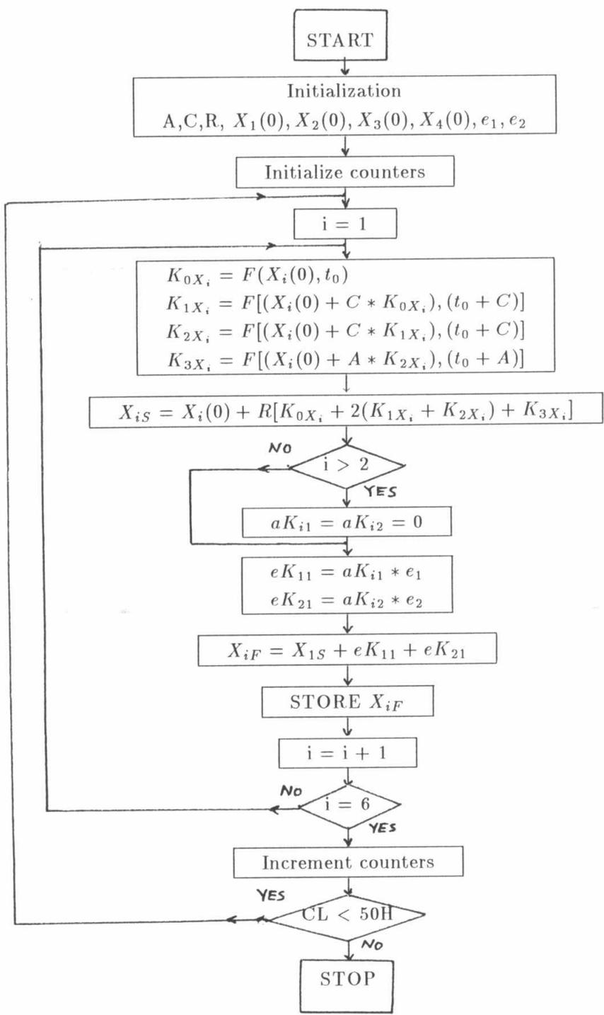
Fig.(5) Flowchart For Calculating State Vector.
