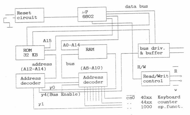
Fig.8. Microprocessor Board
