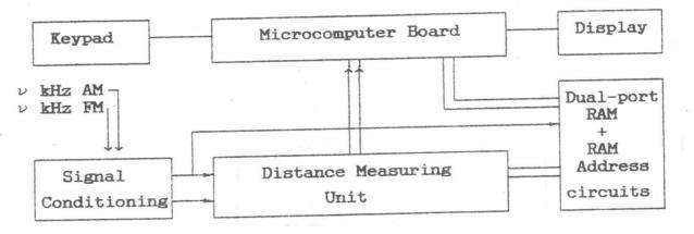
Fig.1.The Digital Processor Functional Diagram
