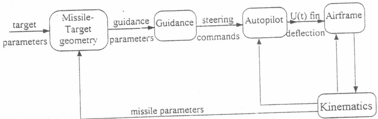
Fig. 3. Simplified block diagram of the main simulation model modules.
