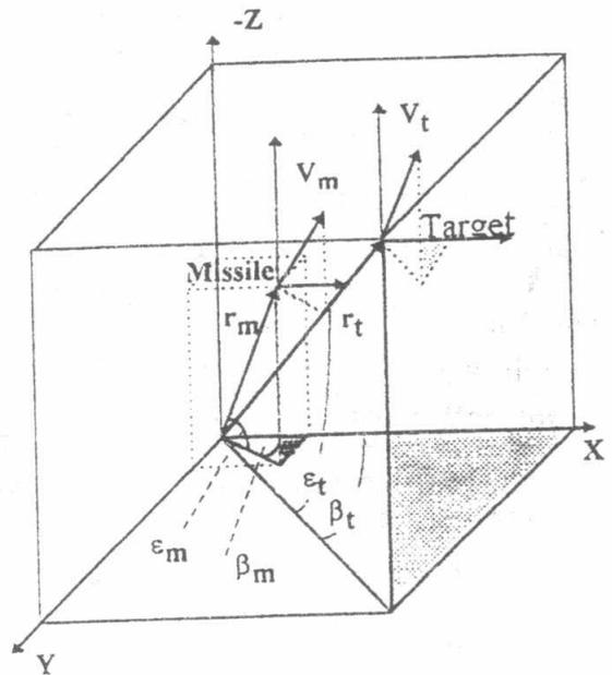
Fig. 1. Simplified block diagram of the guidance system. Fig. 2. Geometry of command guidance system.
