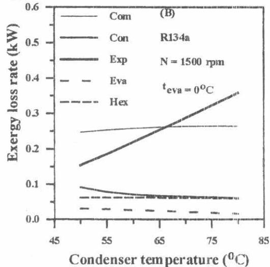
Fig.5 Effect of condensation temperature on specific exergy loss of each component of the VCHP. A at  $T_{eva}=5^{\circ}\text{C}$  and B at  $T_{eva}=0^{\circ}\text{C}$ .
