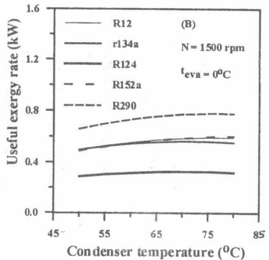
Fig.10 Comparison of useful exergy rate variation for various refrigerants. A at  $T_{eva}=10^\circ\text{C}$  and B at  $t_{eva}=0^\circ\text{C}$ .
