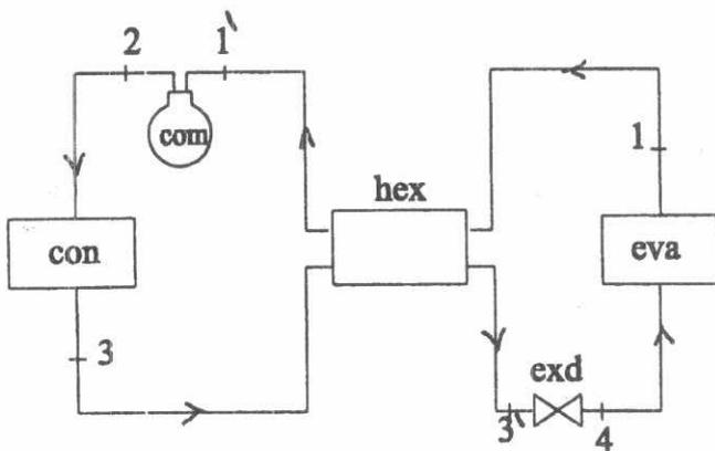
Fig. 1 Schematic diagram of a single stage VCHP.
