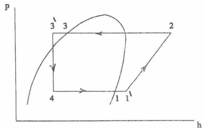
Fig. 2 Pressure-enthalpy diagram of a single stage VCHP.
