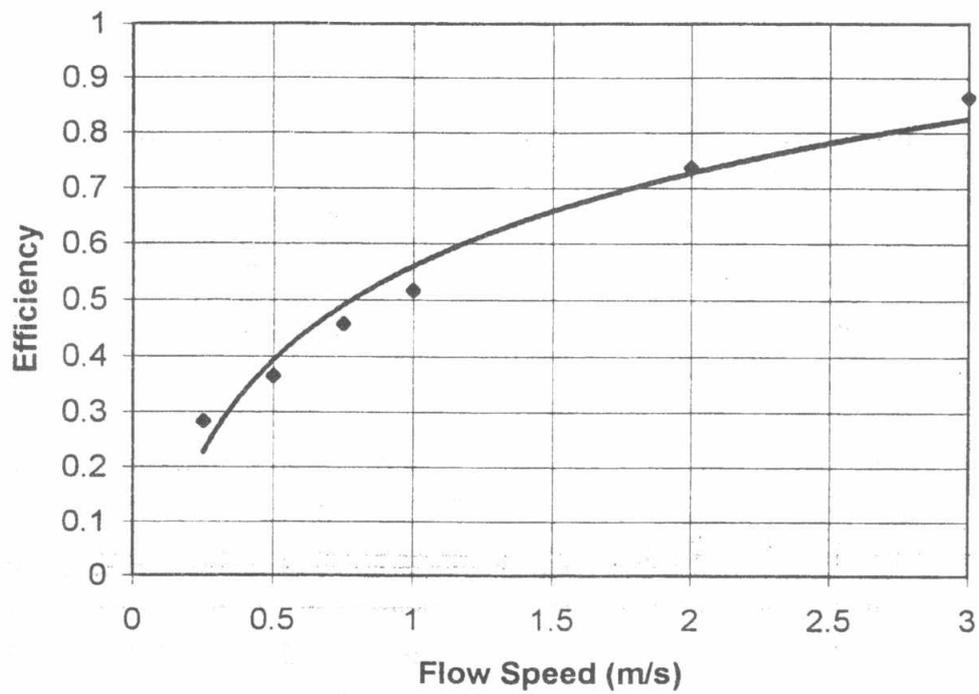
Fig.3 Cyclone Efficiency of Collecting Cement Powder
