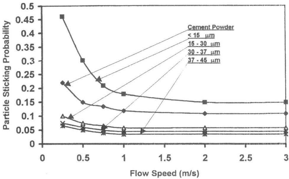
Fig.5 Sticking Probability Versus Flow Speed
