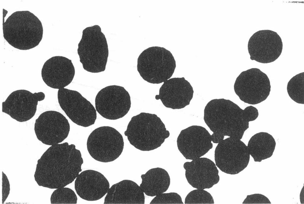
Plate 1 Cement Particles
