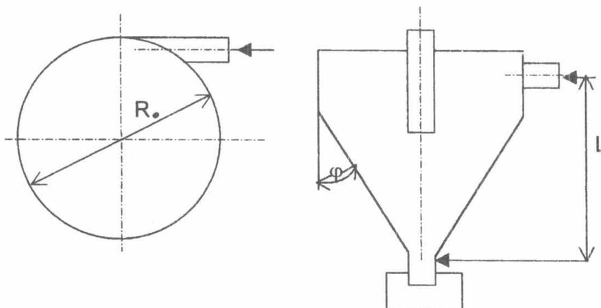
Fig.1. Cyclone Collector
