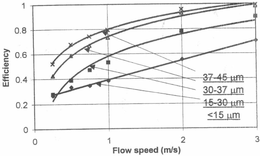
Fig.4 Cyclone Efficiency of Collecting Cement with Different Particle Size
