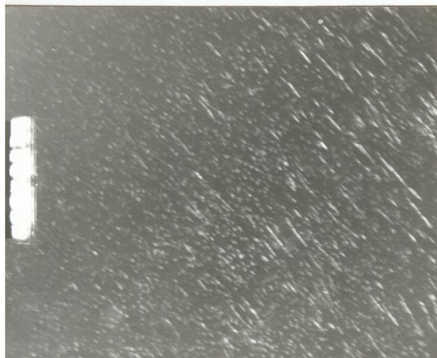
Fig.10 TEM image in dark field, 160000:1-Orthorhombic phase  $\text{Ni}_3\text{Mo}$ , spot (211)
