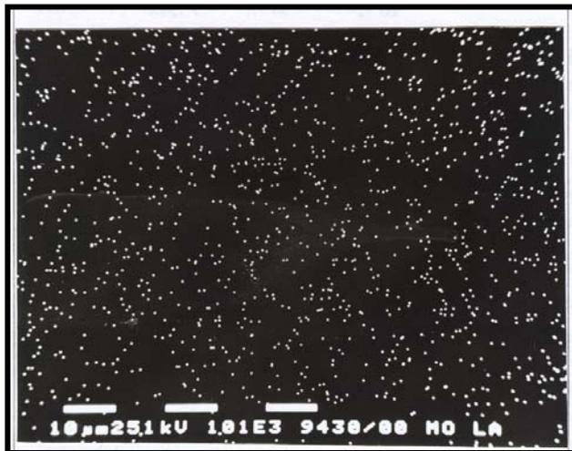
Fig. 5b The image of the distribution of X MoL $\alpha$  rays corresponding to the micro zone in Fig. 5
