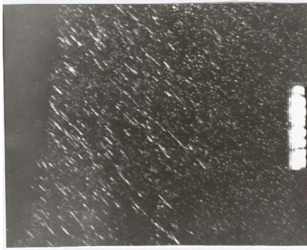
Fig. 11 TEM image in dark field, 160000:1-Tetragonal SIGMA phase  $\text{Ni}_3\text{Mo}$ , spot (022)
